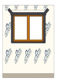
Finish flashing the exterior of the window per QWP nail fin installation guidelines.
