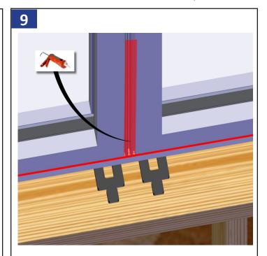
Apply sealant up the bottom 6" of the center of the T-mull filling the entire area as shown above.
