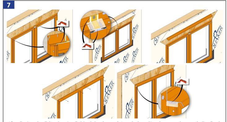
After all units and mulls have been installed, leveled, and squared. Insert backer rod into the top gaps between the T-mull and frames. Apply sealant over the whole top of the T-mull area to cover all gaps between the mull and frame as shown above. Apply a continuous bead of sealant across the entire top outer frame edge then set drip cap and fasten in place. Use backer rod and sealant to cover both ends between the drip cap and frames as shown above.
