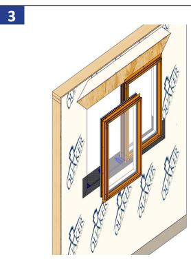
Install the next window unit in place following the QWP standard nail fin installation guide. Make sure the unit doesn't have a nail fin on the side of the unit where the mull will go. Make sure to leave the 1" gap between the units to allow for the T-Mull.
