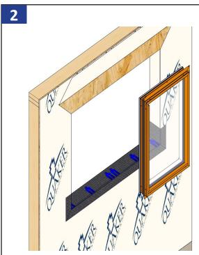
Install the first window unit in place following the QWP standard nail fin installation guide. Make sure the unit doesn't have a nail fin on the side of the unit where the mull will go.
