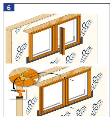
Insert the T-mull centering it between the units from the exterior and fasten with screws.
