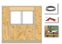
Insert the base plate with weather-strip flat against the window units and install with supplied bolts. Snap the finish trim cap over the base plate to finish the T-mull. Insulate and seal around the entire permiter of the window units.
