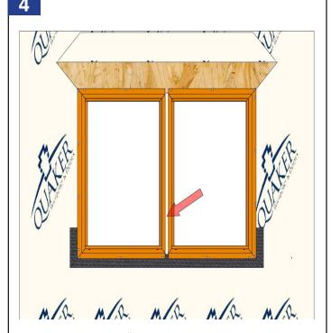
Make sure the gap is 1" between the window units as shown above.
