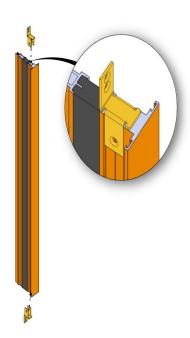
Insert the anchor clips in the top and bottom on the T-mull slots as shown above.
