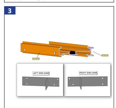
Note the orientation of the stack mull interior and exterior sides. Exterior side will have weep slots. Note orientation for the end dams (left and right as seen from the exterior side of the window).
