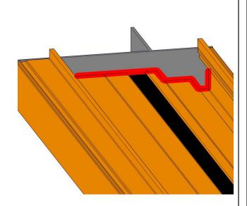
Apply a continuous bead of silicone along the entire inside of
