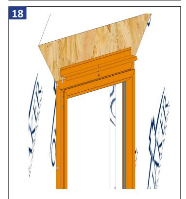
Apply the head flashing to the top edge of window as shown below.
