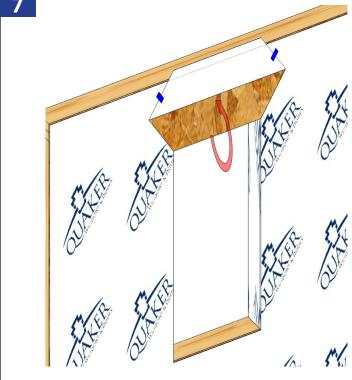
Fold the house wrap flap up and temporarily tape it in place.
