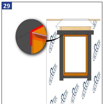
Apply flashing tape over the head flashing, overlapping the side flashing as shown, covering any seam or gap in the nailing fin at the corners. Smooth using a J-roller. Put sealant at top corners of flashing tape.
