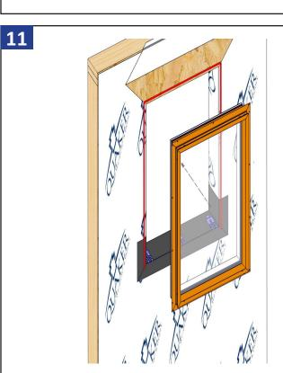
Center the window in the opening, setting the window on the shims. Make sure shims are positioned under each side jamb.
