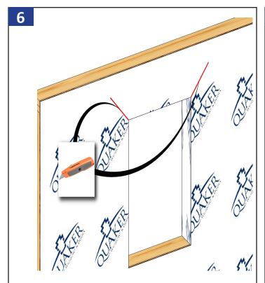
Cut the house wrap to create a top flap as shown. Cut the angles at 45 degrees and  $1^{\prime\prime}$  longer than the width of the flashing tape being used.
