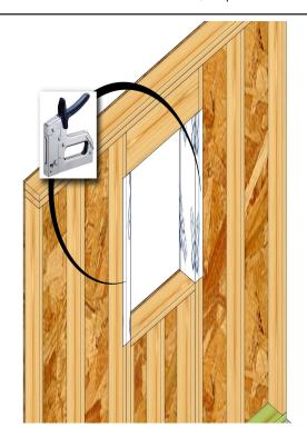
Fold the house wrap to the interior and staple it to the interior framing. Tape the house wrap at the bottom of the opening as shown.
