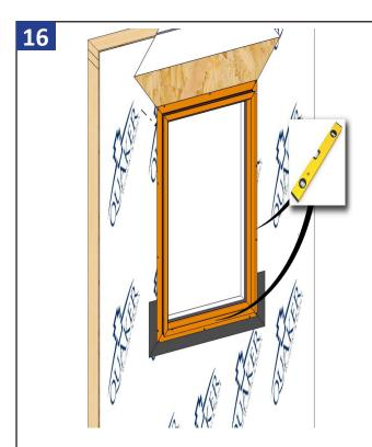
Check that the frame is plumb and level. Adjust shims as needed.
