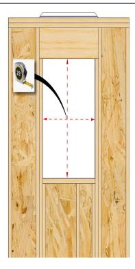
Measure and verify the opening is sized correctly. The rough opening should be a minimum 1/2" (but not to exceed 1") wider and taller than the unit. Allow additional space for flashing thickness, installation clips, joining components, and their fasteners.
