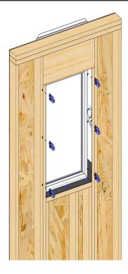
Shim at the sides of the window, and at the check rail locations. Never shim at the head.
