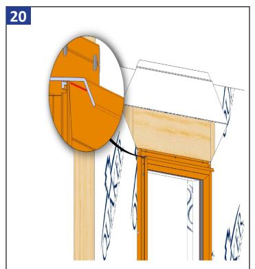
Caulk the seam between the bottom of the head flashing and top of the window.
