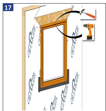
Finish fastening the unit using every hole or a minimum of 12" on center.
