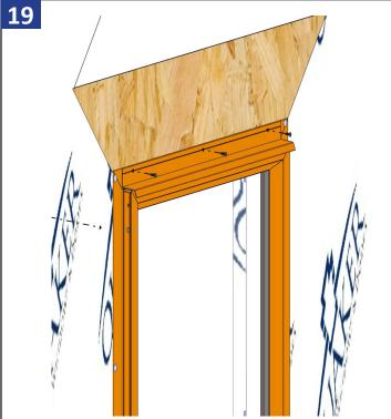
Fasten the head flashing with small self tapping screws. Make sure the head flashing is setting down tight on the window frame.
