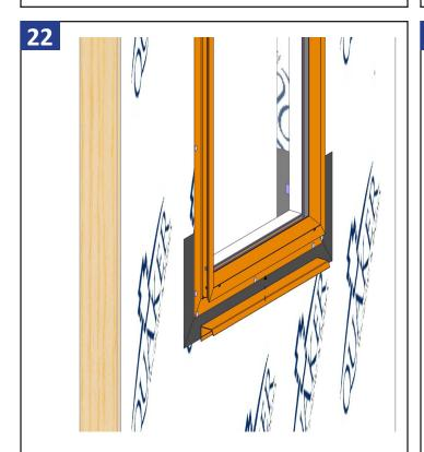
Apply the sill flashing to the bottom edge of window as shown above.
