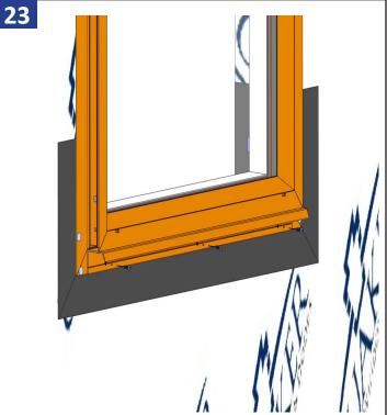
Fasten the sill flashing tight against the bottom of the window with self tapping screws as shown above.
