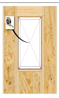
Check that the window is square. Adjust shims as needed to assure unit diagonal measurements are within 1/8".
