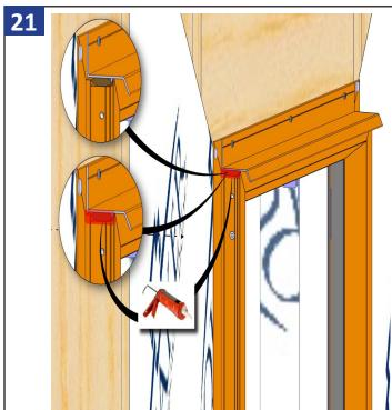
Use backer rod and sealant to seal both ends of the head flashing and window as shown above.
