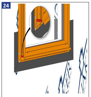
Apply backer rod and sealant to both ends of the sill flashing to seal it against the window as shown above.
