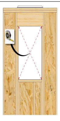
Check that the opening is square. The diagonal measurements need to be within 1/8" of each other.
