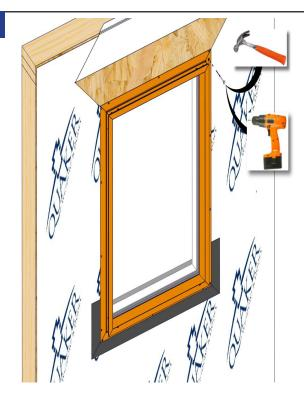
Temporarily fasten with a single fastener at the top of one jamb side as shown.
