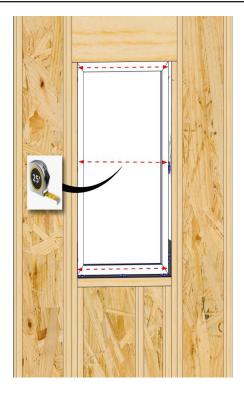
Check that the window is not bowed. Adjust shims as needed unit measurements are within 1/8".
