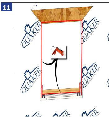
Apply a continuous 3/8"sealant bead at the sides and the top of the opening, no more than 1/2" from edge of opening as shown. **Sealant needs to line up nail hole slots**. If using QWP sill pan flashing system apply a continuous 3/8" sealant bead to the inside up turned leg for the window to set against when installed.
