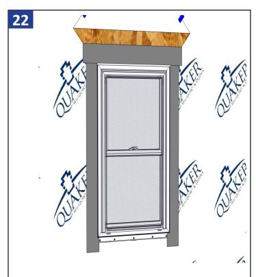
Unfold the house wrap top flap and tape the angled seams
