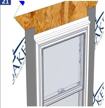
Place the drip cap the full width in sealant as shown.
