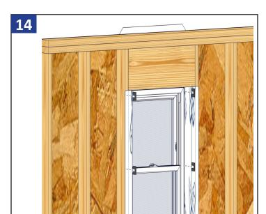
Shim at the sides of the window, and at the check rail locations. Never shim at the head.
