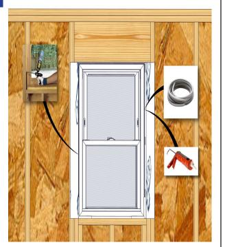
Apply sealant continuously around entire perimeter of opening, filling interior 1/3 of cavity using low expanding foam or backer rod and sealant.
