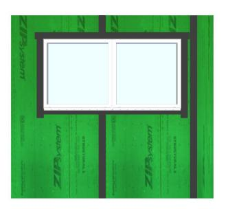
Apply a 3/8" sealant bead to the top exterior edge of window frame before installing the drip cap. Cut a piece of flashing tape for the head flashing, which extends beyond outer edges of jamb flashings. Tape any other vertical seams above the window making sure to lap the tape a minimum of 1" over the head flashing.
