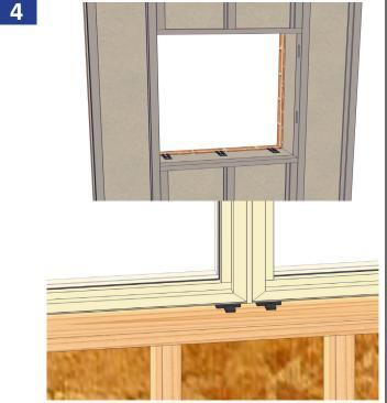
Place shims on the bottom of the opening under each side jamb location insert 1/4" from each side. If installing a mulled unit make sure to shim at all mull locations as shown above.
