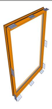
Slide the anchor straps onto the interior C-leg of window frames as shown above. Locate the anchor straps around the entire window perimeter positioned as noted on the shop drawings and or anchorage calculations. Typically 3" from the corners and 12" on center.
