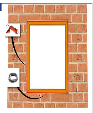
Apply backer rod and a continuous minimum 3/8" bead of sealant around the entire perimeter of the opening.
