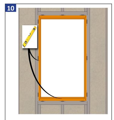
Check that the frame is plumb and level. Adjust shims as needed.
