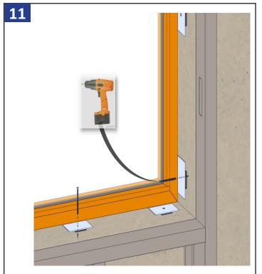
Finish fastening the unit using a minimum of one screw per anchor strap.
