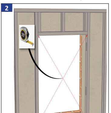
Check that the opening is square. The diagonal measurements need to be within 1/8" of each other.
