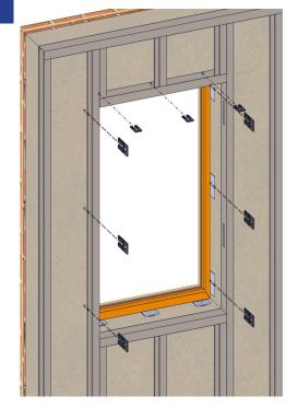
Shim at the sides of the window, and the check rail locations. Make sure to shim the window and the backside of the anchor straps.
