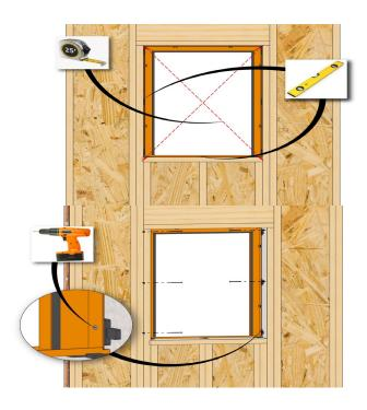
Measure the Masonry opening and trim panning legs as needed to fit openings. Shim as needed to square, plumb, and level the panning into the opening. Fasten the panning with screws by others per shop drawings or anchorage calculations. Typically 3" from the corners and 12" on center. Always follow the fastener/anchor manufacture's guidelines for proper edge distance, load capacity and installation techniques.
