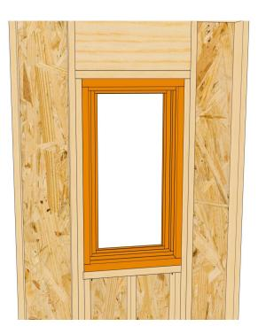
Insulate between the window frame and the rough opening using minimally expanding window and door spray foam or fiberglass insulation that is compliant with AAMA 812-04. Read and follow the manufacturers' recommendations for application and use. Install the snap trim covers to finish the interior.
