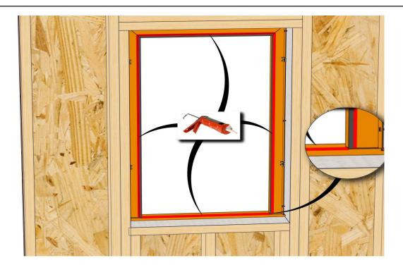
Apply a continuous bead of sealant along the sill panning where the exterior window leg will rest. Back bed the panning vinyl with sealant just before insertion of the window, or cap seal the window to the panning frame joint from the exterior after the window is installed. Whichever method is used, the window must be wet sealed to the panning. The panning vinyl is not an adequate weather seal. Insulate around perimeter between the panning and wall system.
