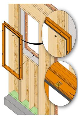
Install the clips per above image if not done at the factory. Check the fit of the panning making sure the conditions are level.
