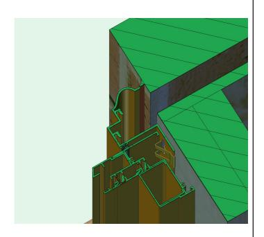
Set the exterior leg of the window onto the sill panning frame. Then push the window head and jamb in against the panning head and jamb. Make sure that the window head and jamb legs snap-in securely behind panning clips. The window must be pushed tight against the panning.
