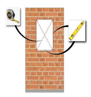
Measure and verify the size of the rough opening. See shop drawings for the proper opening sizes per panning system being used. Verify the rough opening is flat, plumb, level, and square. Take diagonal measurements to check for square. The sill beneath the unit must be level for proper unit operation.
