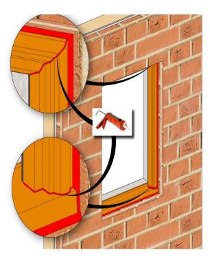
Apply sealant to the perimeter of the panning system to the surrounding masonry opening, and all seams in the panning system.
