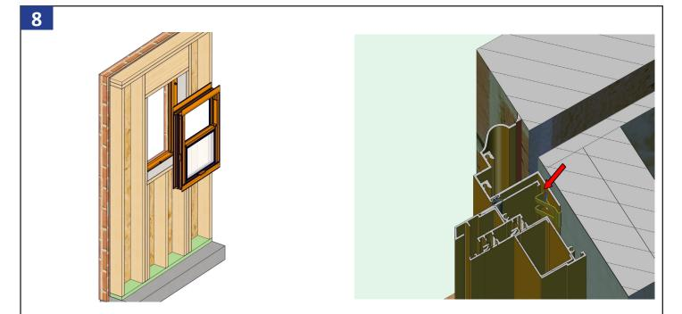
Set the exterior leg of the window onto the sill panning frame. Then push the window head and jamb in against the panning head and jamb. Make sure that the window head and jamb legs snap-in securely behind panning clips. The window must be pushed tight against the panning.
