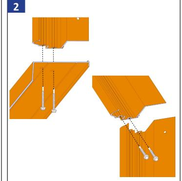
Assemble sill panning to panning jambs, and jambs to panning head using two of the supplied screws at each corner. Screw through the holes in sill and jambs into the screw bosses.
