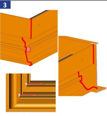
Back seal all four outside corners of the panning. Completely cover the miters, screw heads and exposed screw bodies with sealant.
