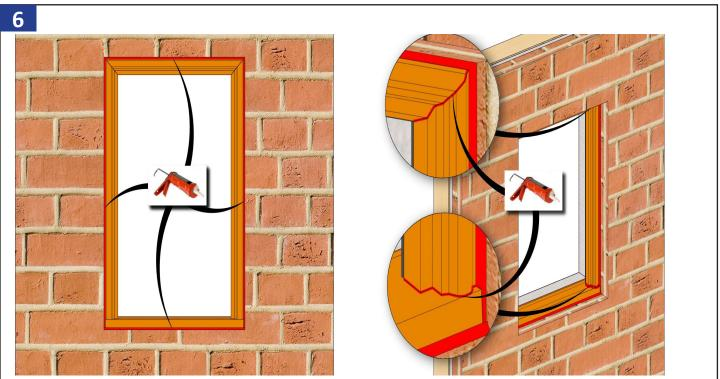
Apply sealant to the perimeter of the panning system (3/8" caulk joint) to the surrounding masonry opening, and all seams in the panning system.
