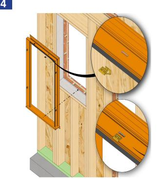
Install the panning clips (shipped separately from panning) per the above image. Check the fit of the panning making sure the conditions are level and shim as needed to achieve level.
