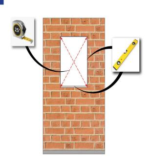
Measure and verify the size of the rough opening. See shop drawings for the proper opening sizes per panning system being used. Verify the rough opening is flat, plumb, level, and square. Take diagonal measurements to check for square within 1/8". The sill beneath the unit must be level for proper unit operation.
