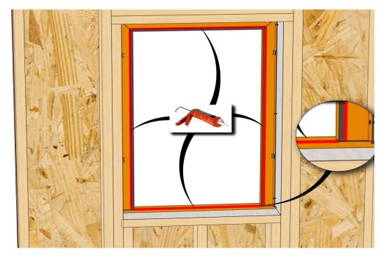
Apply a continuous bead of sealant along the sill panning where the exterior window leg will rest. Back seal the panning vinyl with sealant just before inserting the window, or cap seal the window to the panning frame joint from the exterior after the window is installed.
