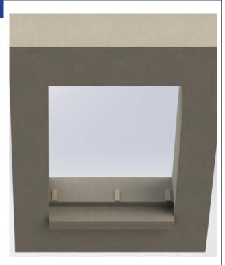
Check the fit of the unit making sure the conditions are level, the installer can pre-apply the shims to the sill condition prior to installation of the window frame.
