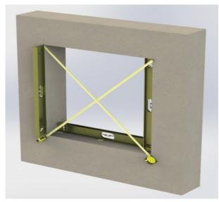
Measure and verify the size of the rough opening. The rough opening should be a minimum %" (but not to exceed 1") wider and taller than the unit. The masonry opening should be sized %" wider and 9/16" higher than the units exterior frame. Verify the rough opening is flat, plumb, level, and square. Take diagonal measurements to check for square.
