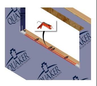
Apply a continuous beads of sealant on the sill and exterior wall face between the corners as shown above.
