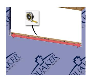
Measure between the two corner molds and cut the sloped section 1" less to allow for the curves in the corners.
