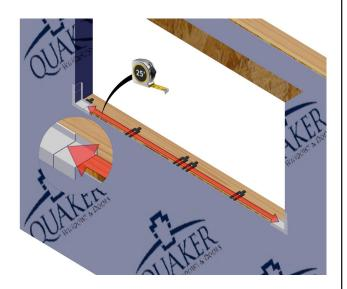
Measure and cut the center sill flashing section. Cut the side that has the 4" notch so you have at least 2" of overlap on each side. Dry test fit to make sure everything will fit together with the proper flush overlaps before the next step.
