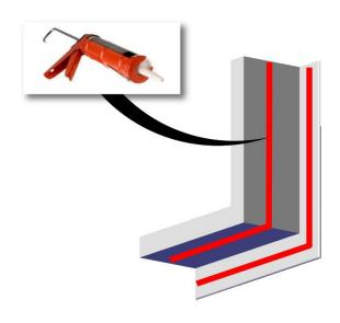
Apply a bead of sealant on each the back and bottom smooth (non-stepped) sides of the corners as shown above.
