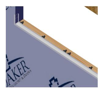
Set center flashing section in place pressing firmly to allow cement to bond.
