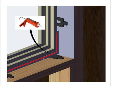
Apply a bead of sealant to fill the gap between the sill pan flashing system and the window unit.
