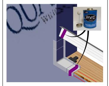
Clean the ends before applying PVC cement to both ends of the center and both corners.
