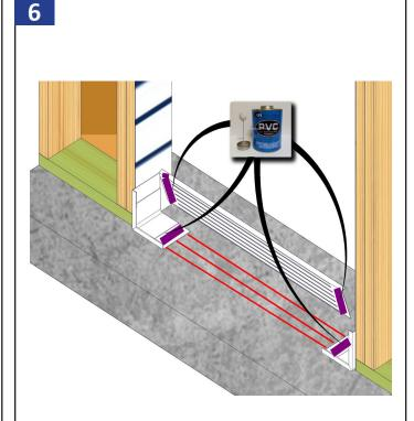
Clean the ends before applying PVC cement to both ends of the center and both corners.
