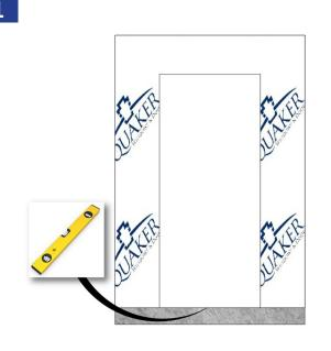
Measure and verify the size of the rough opening. See shop drawings for the proper opening sizes. Verify the rough opening is flat, plumb, level, and square. The sill beneath the unit must be level for proper unit operation. Check the fit of the sill pan system making sure the conditions are level, the installer can pre-apply the shims to the sill condition prior to installation of the sill pan flashing system.
