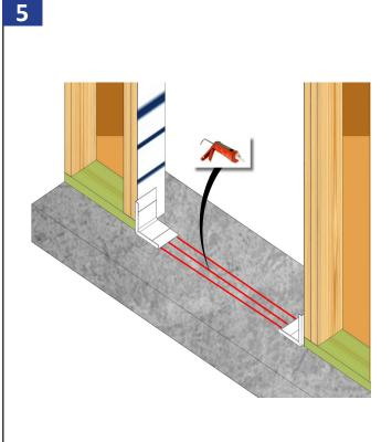
Apply three continuous beads of sealant on the sill between the corners.
