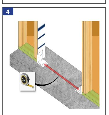
Measure and cut the center sill flashing section. Cut the side that has the 4" notch so you have at least 2" of overlap on each side. Dry test fit to make sure everything will fit together with the proper flush overlaps and that the sill is level.
