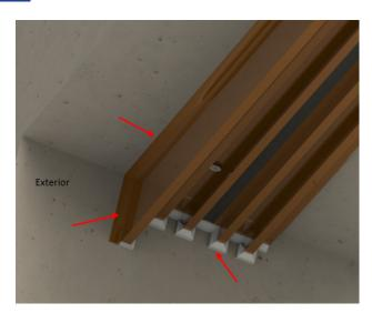
Shim as needed to level head receptor before tightening all screws.
