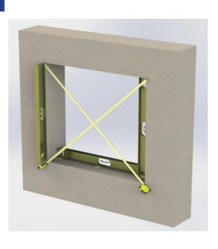
Measure and verify the size of the rough opening. See shop drawings for the proper opening sizes per sub-sill and receptor system being used. Verify the rough opening is flat, plumb, level, and square. Take diagonal measurements to check for square. The sill beneath the unit must be level for proper unit operation.
