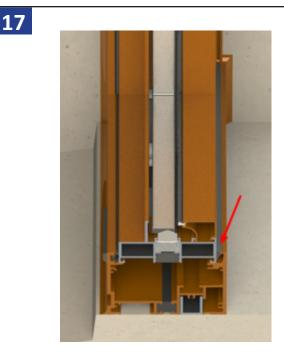
Place a level on the window sill to verify that the sill is level. Adjust the shims as needed to ensure a level condition. Apply the sub-sill wedge gasket into the interior side of the sub-sill against the window as shown above.
