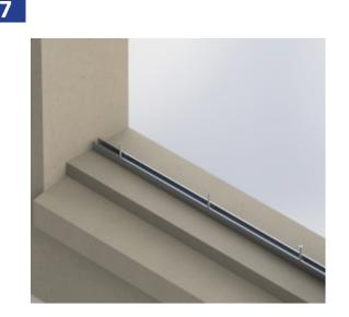
Pre-drill holes and fasten the U-channel with screws by others per shop drawings or anchorage calculations. Typically 3" from the ends and 12" on center.
