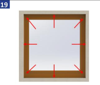
Measure between the sub-sill and head receptor clip and cut the jamb receptor closer clips. Trim weather strip to appropriate length using caution not to stretch material. Install clip using a rubber mallet to make sure the closer clip snaps into place.
