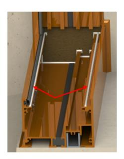
Apply a bead of sealant to the legs of the sub-sill where the window will rest. Center window in opening and set the exterior leg of the window onto the sub-sill frame, then push the window head and jamb in against the head and jamb receptors. Snap in temporary closer pieces to hold window into place.
