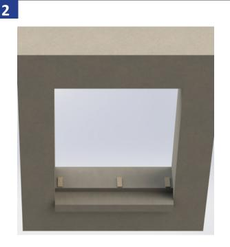
Check the fit of the sub-sill making sure the conditions are level, the installer can pre-apply the shims to the sill condition prior to installation of the sub-sill.
