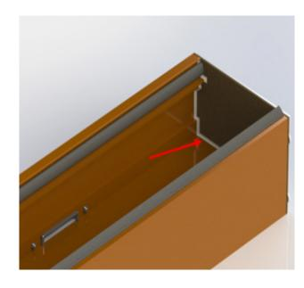
Apply self-leveling sealant to the inside edge between the sub-sill and the end dam covering all edges.
