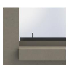
If flashing is present, determine where the window will be positioned to ensure that the perimeter seal is inboard of the flashing so water drainage will occur outboard of the perimeter joint at the head receptor.
