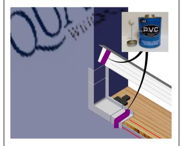
Clean the ends before applying PVC cement to both ends of the center and both corners.
