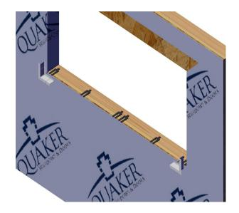
Install the corner molds into both corners making sure they are tight against the rough opening and shimmed sill.
