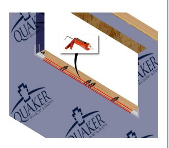
Apply a continuous beads of sealant on the sill and exterior wall face between the corners as shown above.
