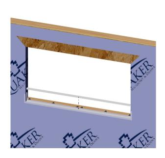
Install sloped section making sure the ribs on the bottom lock into the ribs on the center sections.
