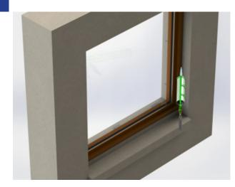
If total frame replacement in brick or siding was preformed maintain a minimum of %" between the window frame, trim, siding, or masonry. Failure to do so could result in product or property damage. Apply backer rod (if needed) and a continuous bead of sealant between the window frame and exterior finish material on all four sides of unit. Make sure to clean all surfaces before applying 100% neutral cure silicone sealant (some surfaces may need to be primed so check with sealant supplier).
