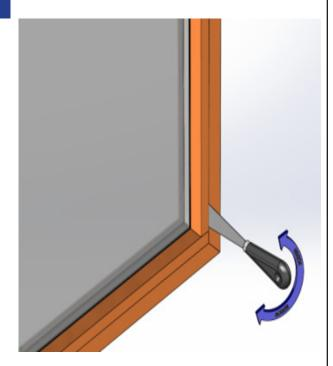
The glazing bead may require removal and reinstallation. Be careful to avoid damaging the glazing beads and finish. Slide a putty knife between the glazing bead and frame at the bottom corner and apply pressure as you rotate the putty knife away from the window frame.
