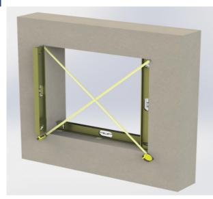
Measure and verify the size of the rough opening. The rough opening should be a minimum  $\frac{1}{2}$ " (but not to exceed 1") wider and taller than the unit. The masonry opening should be sized  $\frac{1}{2}$ " wider and  $\frac{9}{16}$ " higher than the units exterior frame. Verify the rough opening is flat, plumb, level, and square. Take diagonal measurements to check for square.
