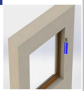
Insulate between the window frame and the rough opening using minimally expanding window and door spray foam or fiberglass insulation that is compliant with AAMA 812-04. Read and follow the manufacturers' recommendations for application and use.
