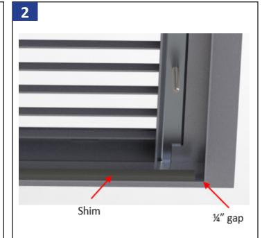
Insure that the  $\frac{1}{2}$  x  $\frac{3}{16}$  shim is in place across the bottom. Trim corners  $\frac{1}{2}$  from the ends to allow for sealant.
