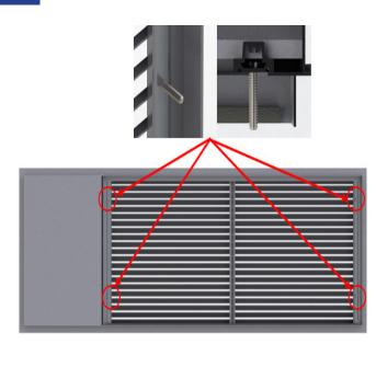
Locate and install sleeve mounting studs (if not already in place). Inspect perimeter sealing flange and clean per sealant manufacturers recommendations.
