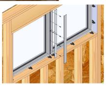
Apply sealant up the bottom 6" of the center of the T-mull filling the entire area as shown above. Insert the base plate with weather-strip flat against the window units and install with supplied bolts.
