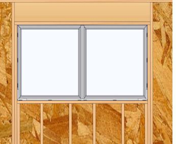
Snap the mull cover plate over base plate to finish off interior mull.
