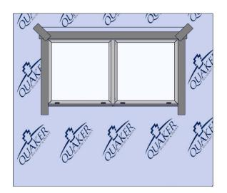
Finish flashing the exterior of the window per QWP nail fin installation guidelines.
