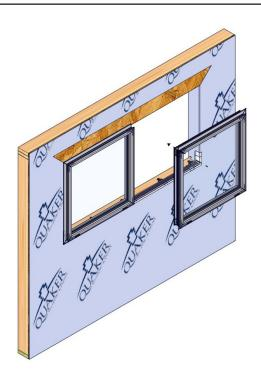
Install the next window unit in place following the QWP standard nail fin installation guide. Make sure the unit doesn't have a nail fin on the side of the unit where the mull will go.
