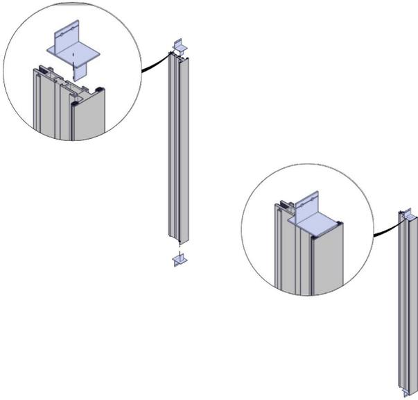
Insert the Z. clips in the top and bottom on the T-mull slots as shown above.
