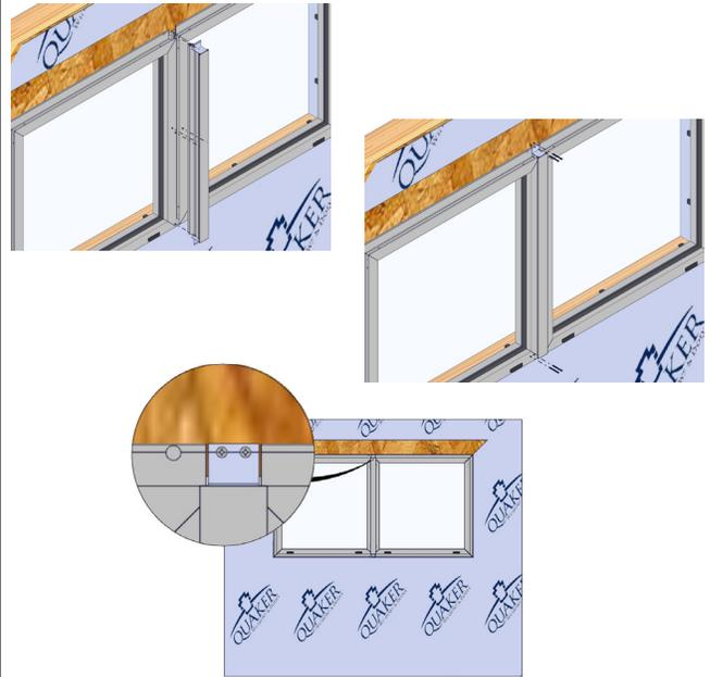
Insert the T-mull centering it between the units from the exterior and fasten with screws.
