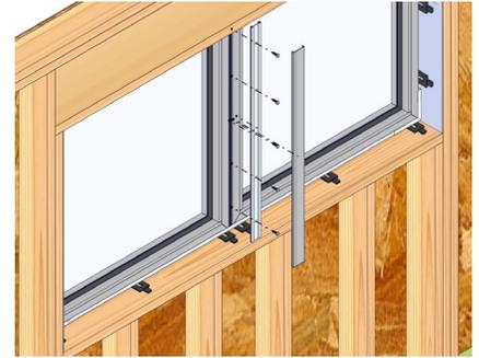
Apply sealant up the bottom 6" of the center of the T-mull filling the entire area as shown above. Insert the base plate with weather-strip flat against the window units and install with supplied bolts.
