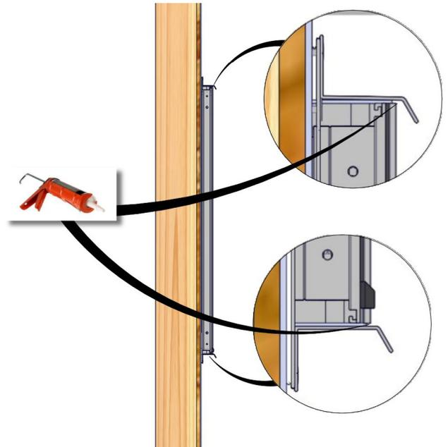
Apply a continuous bead of sealant to seal the drip cap to the windows.
