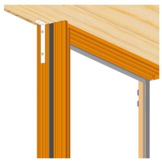
**For Install Without Nail Fins:** L-angles will be used in place of anchor clips and are installed after the first unit. Verify T-mull is vertical and centered properly between the units being installed.
