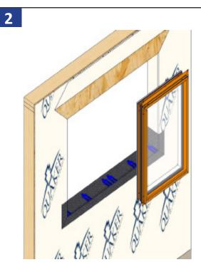
Install the first window unit in place following the QWP standard nail fin installation guide. Make sure the unit doesn't have a nail fin on the side of the unit where the mull will go.
