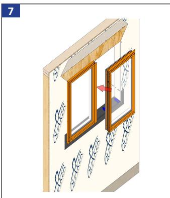
For Install Without Nail Fins: Install the next window unit in place following the appropriate Quaker installation guide. Make sure the unit doesn't have a nail fin on the side of the unit where the mull sits. Window units should be 1" apart
