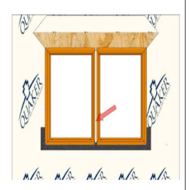
Install the next window unit in place following the QWP standard nail fin installation guide. Make sure the unit doesn't have a nail fin on the side of the unit where the mull will go. Make sure to leave the 1" gap between the units to allow for the T-Mull as shown.
