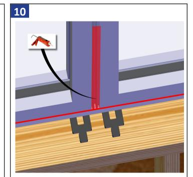
Apply sealant up the bottom 6" of the center of the T-mull filling the entire area as shown above.
