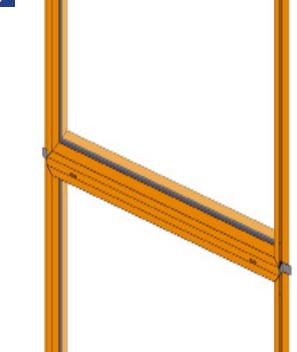
Shim, adjust and secure units in the opening per the QWP standard nail fin installation guide.
