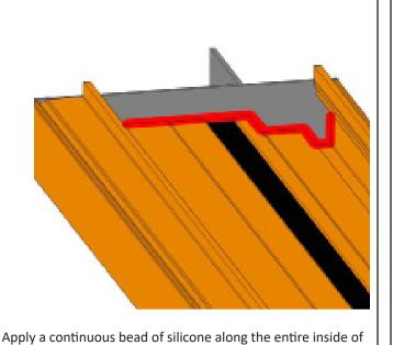
the edge of the end dam following the contour of the mull.
