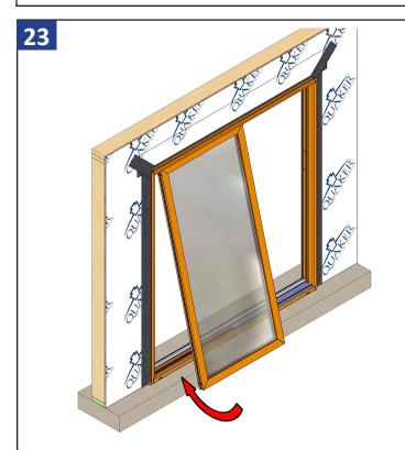
Angle the fixed panel with the top inserted into the head track, and then lift and set the bottom of the panel on the fixed panel extrusion in the sill.
