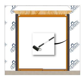
Apply flashing tape at the sides of the door as shown. Smooth using a J-roller. Extend tape a minimum of 2" past door frame, but not more than the thickness of the flashing tape.
