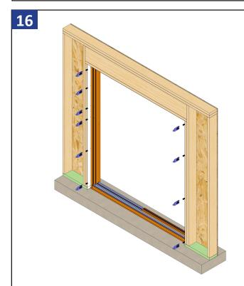
Shim at the sides of the door, and at the lock location as shown above. Never shim at the head.
