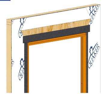
Apply a 3/8" sealant bead to the top exterior edge of door frame before installing the drip cap.
