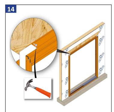
Temporarily tack the door into place using 2" galvanized roofing nails through the pre-punched holes on one top corner of the nailing flange.
