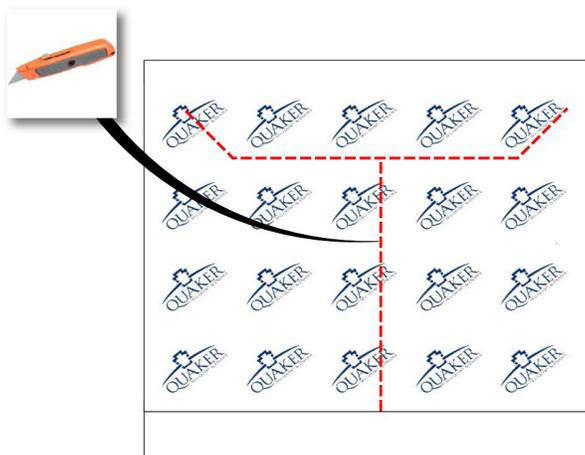
Apply the house wrap according to the manufacturer's instructions and cut T-pattern opening as shown. Cut top flap angles at 45 degrees and 1" longer than the width of flashing tape being used.
