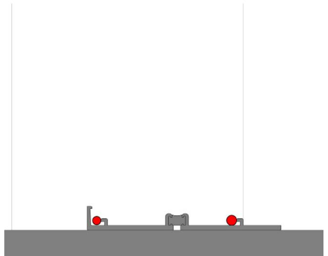
Run a continuous bead of sealant along each leg the entire width.
