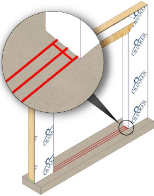
The sub-sill anchor plate will set  $4 \frac{1}{16}$ " in from the exterior face of wall framing. Apply three  $\frac{3}{8}$ " continuous beads of sealant across the entire width of the rough opening sill where the sub-sill anchor plate will set. Apply two  $\frac{3}{8}$ " continuous beads the depth of the anchor plate,  $\frac{1}{2}$ " from each side of opening as shown above.
