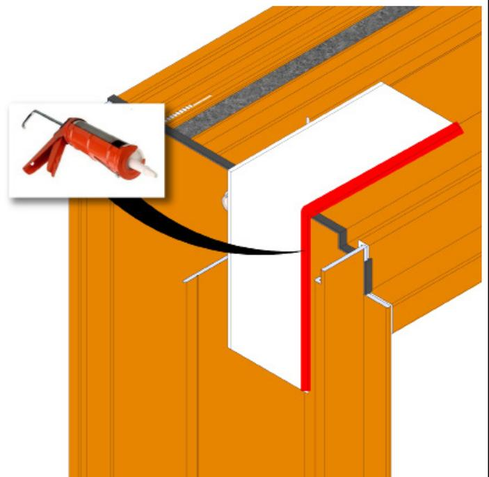
Clean the nail fin corners with 99% isopropyl alcohol prior to installing the aluminum corner to the exterior side of nail fin corner gaps. Apply sealant along the edge where the gasket meets the door frame as shown.
