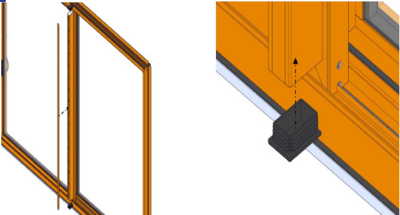
Install reinforcing cover and end caps to reinforcing tube.
