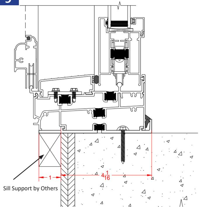
Install the sub-sill anchor plate  $4 \frac{1}{16}$ " in from the exterior face of wall framing. The unit must be supported the full width and depth of the sill.
