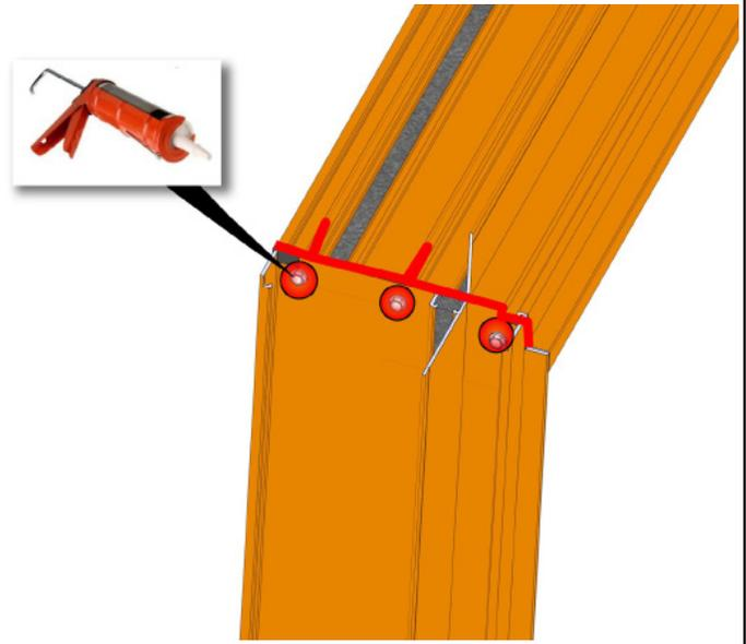
For KD and pre-assembled frames, seal around all screw heads, exposed screw threads, and outside corners.
