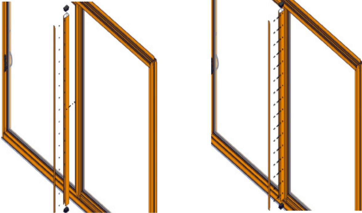
If reinforcing tube is to be applied, center the reinforcing tube on the active panel's meeting rail, and install using supplied (MH8-18x1/2 TK2) screws.
