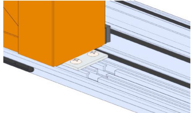
For M204 units, install the meeting rail using supplied (MH8-18X1/2 TK2) screws in the head, and (MP10/24X3/8 & 10-24 NUT) screws and nuts in the sill angle brackets.
