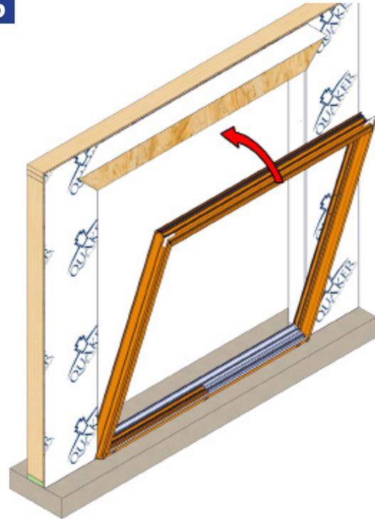
Center and set the door frame into the rough opening, making sure there are equal gaps on both sides of the door.
