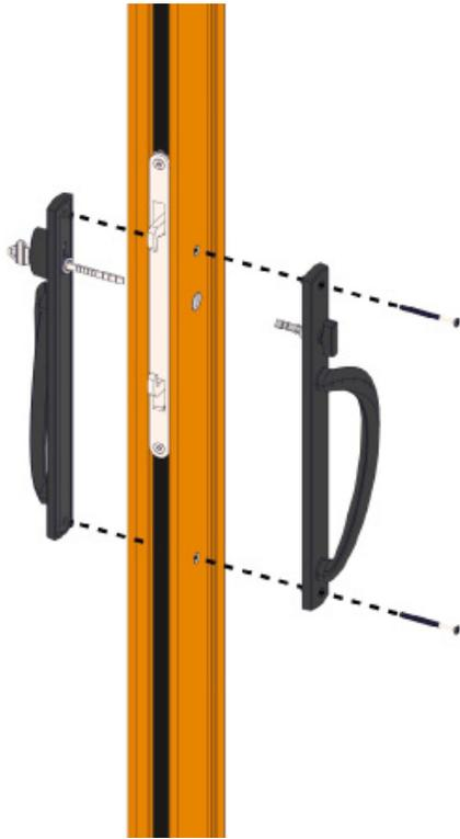
Install handle set using provided instruction found in the hardware box using the 1 7/8" door thickness section.
