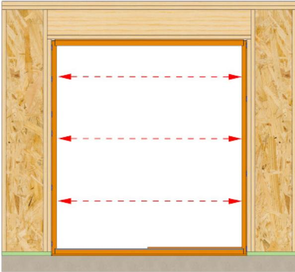
Check that the door frame is not bowed. Adjust shims as needed until measurements are within 1/8". Finish fastening the unit every hole or a minimum of 12" on center.
