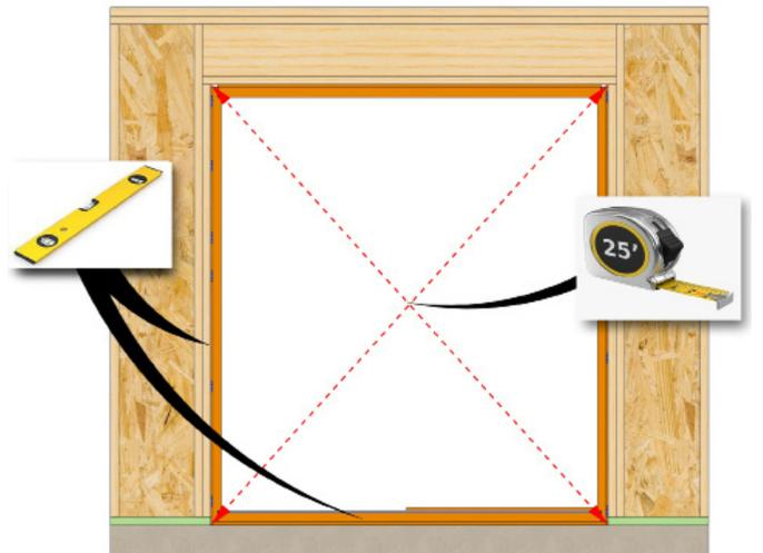
Check that the door is square. Adjust shims as needed until diagonal measurements are within 1/8". Level at the sill and plumb the frame.
