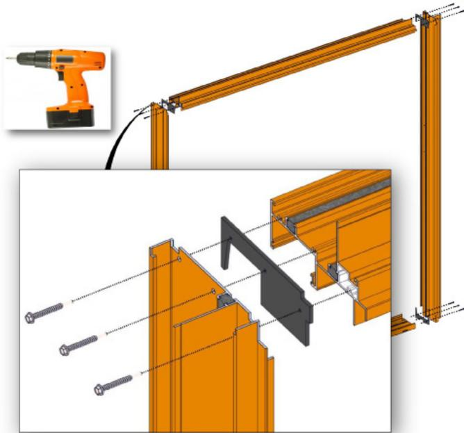
Apply the head and sill gaskets to each end of the head and sill. Assemble jambs to head and sill assembly with the 12 fasteners provided (MH8-18X11/2 LP) Install the jamb with the door keeper holes to the side of the sill that does not have the fixed panel adapter.
