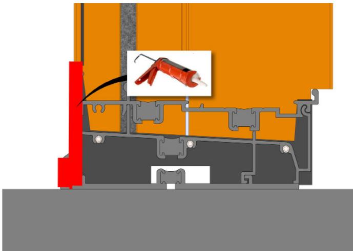
After install take silicone to end dam each side of the sill.
