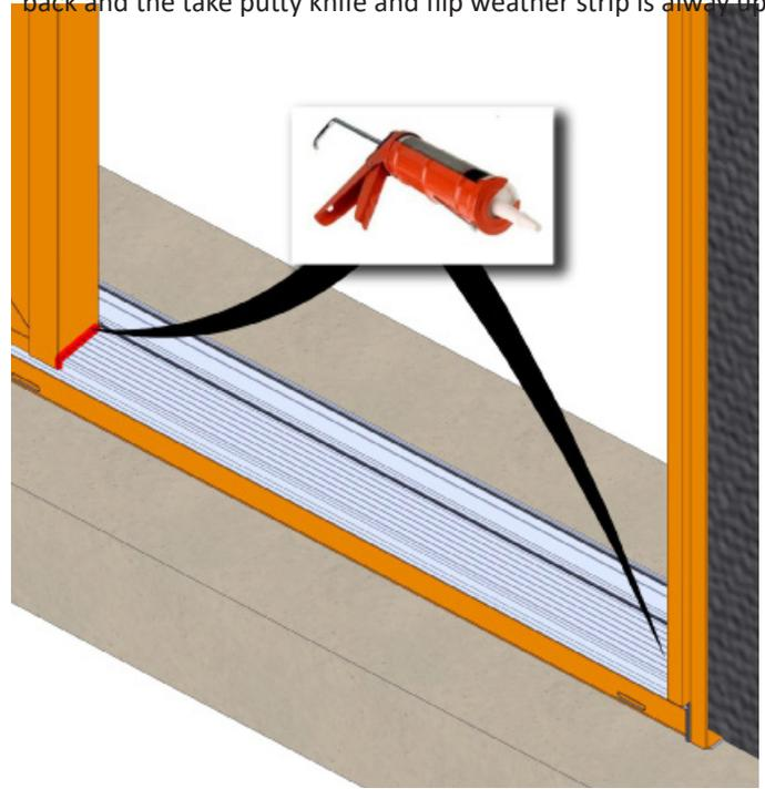
Install threshold on the exterior side of frame covering the bottom angle brackets. Seal around the two ends of the threshold against the frame as shown above.
