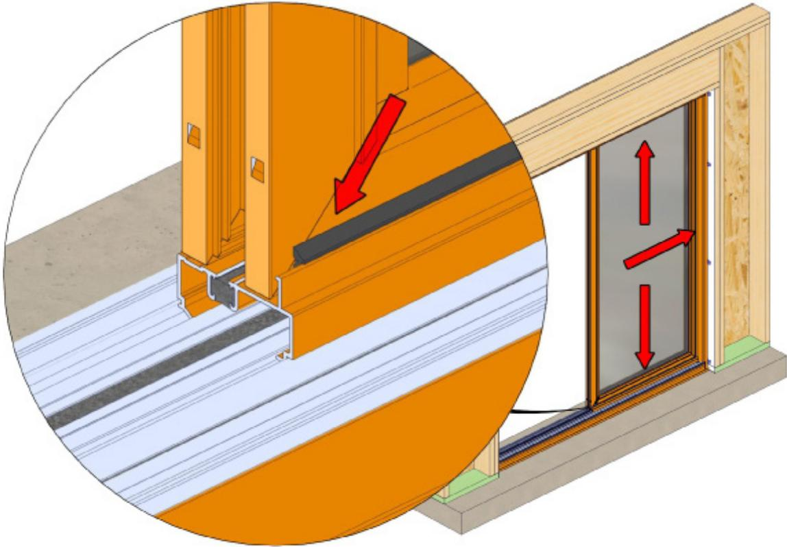
Install wedge gaskets in the sill, head, and jamb around the interior of the frame and panel to secure the panel in place.
