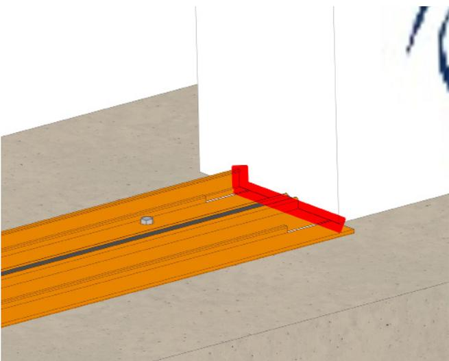
Be sure to run a bead of silicone across the plate and up the interior leg as shown above.
