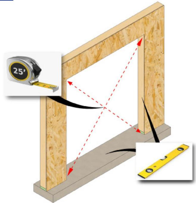
Check that the opening is square. The diagonal measurements need to be within  $1/8$ " of each other. Verify the rough opening is plumb and level. **The sill plate beneath the unit must be level for proper unit operation.**
