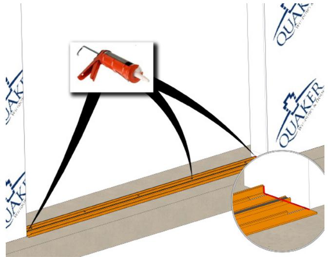
Apply sealant over fastener heads and at the ends of the sub-sill anchor plate where the plate meets the wall framing.
