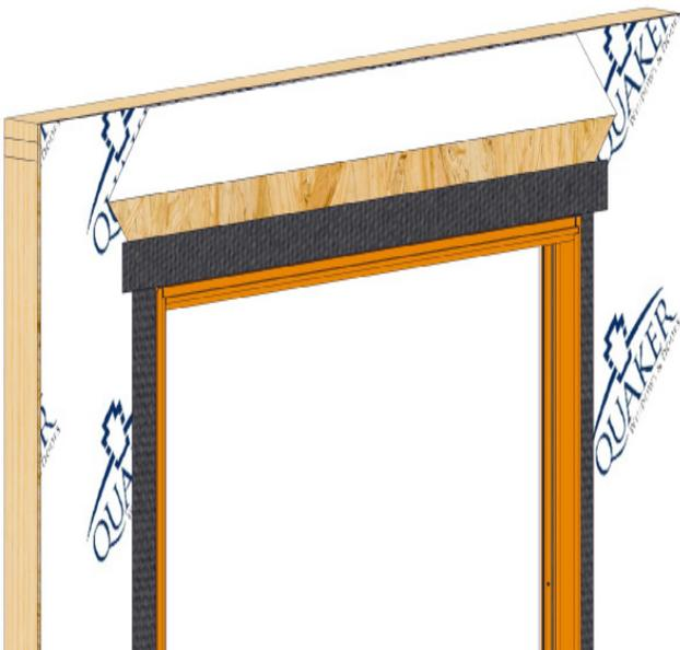
Apply a 3/8" sealant bead to the top exterior edge of door frame before installing the drip cap. Apply flashing over the drip cap leg, overlapping the side flashing as shown. Smooth using a J-roller.
