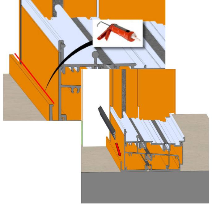
Run a bead of silicone along the joint prior to installing the wedge gasket in the sub-sill anchor plate against the interior leg of the door as shown above.
