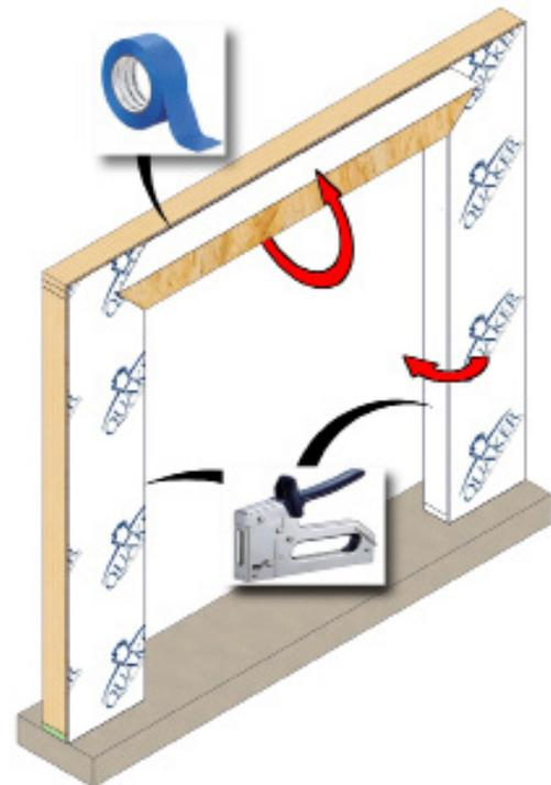
Fold the house wrap around the jambs to the interior and staple it to the interior framing. Fold the house wrap flap up and temporarily tape it in place.
