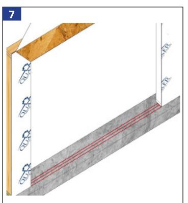
Apply three 3/8'' continuous beads of silicone across the entire width of the rough opening sill, and a 3/8'' continuous bead of silicone  $\frac{1}{2}''$  from each side of the rough opening as shown above.
