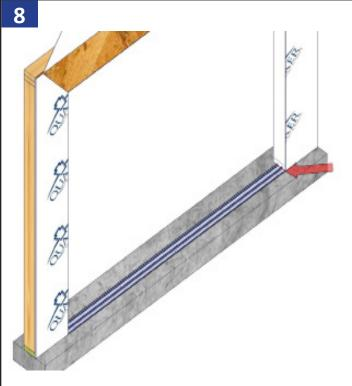
Install the sub-sill anchor plate keeping the exterior edge of sub-sill anchor plate in line with exterior of wall framing.
