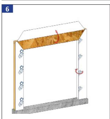
Fold the house wrap to the interior and staple it to the interior framing. Fold the house wrap flap up and temporarily tape it in place.
