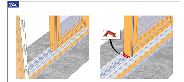
For all other M-Series units, install the pre-assembled meeting rail against the fixed panel and install using supplied (MH8-18X1/2 TK2) screws in the head and sill angle brackets.
