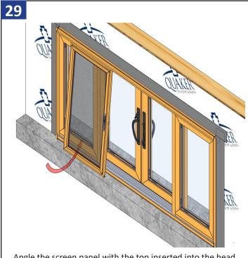
Angle the screen panel with the top inserted into the head track, and then lift and set the bottom rollers on the roller track. Adjust rollers as needed to insure the panel is level, square, and slides smoothly. Repeat above steps for the other screen.
