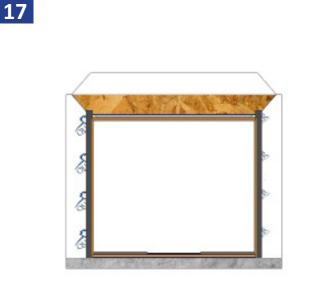
Apply flashing tape at the sides of the door as shown. Smooth using J-roller. Extend tape a minium of 2" pass window frame.
