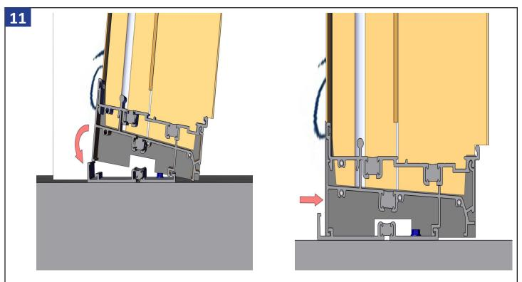
Center and set the door frame into the rough opening, making sure there are equal gaps on both sides of the door. Angle the door frame with the top tilted out, and set the exterior sill frame inside the exterior leg of the sub-sill anchor plate. Push the frame in against the framing locking the sill into the sub-sill anchor plate.
