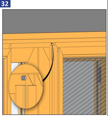
Install a stop screw into the head frame to keep screens centered when locked.
