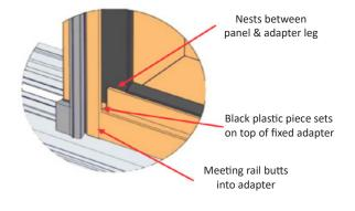
Apply a bead of sealant to inside edges of meeting rail before sliding the pre-assembled meeting rail against the fixed panel. Please see steps 24b and 24c for series specific guidelines.
