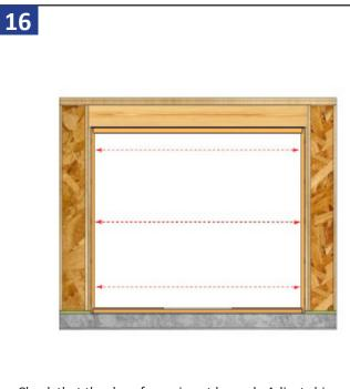
Check that the door frame is not bowed. Adjust shims as needed until measurements are within 1/8". Finish fastening the unit every hole or a minium of 12" on center.
