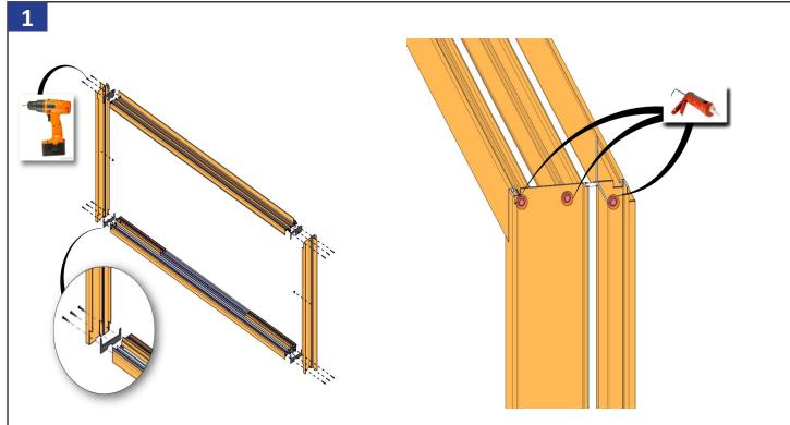
Assemble jambs to head and sill assembly with the 12 fasteners provided (MH8-18X11/2 LP). Make sure to use the two head and sill gaskets provided, and seal around screw heads and outside corners.
