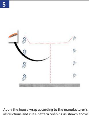
Apply the house wrap according to the manufacturer's instructions and cut T-pattern opening as shown above. Cut top flap angles at 45 degrees and 1" longer than the width of flashing tape being used.
