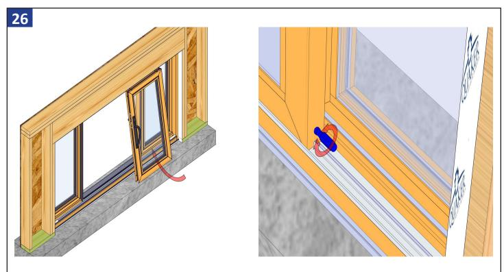
Angle the active panel with the top inserted into the head track, and then lift and set the bottom rollers on the roller track. Use a Phillips #3 screwdriver to adjust the rollers as needed to ensure the panel is level, square, and slides smoothly. Lift on the panel while adjusting, do not use a drill to adjust. Repeat above steps for the other active panel.
