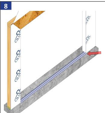
Install the sub-sill anchor plate keeping the exterior edge of sub-sill anchor plate 1" past the exterior of wall framing.
