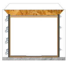
Apply flashing tape at the sides of the door as shown. Smooth using J-roller. Extend tape a minium of 2" pass window frame.
