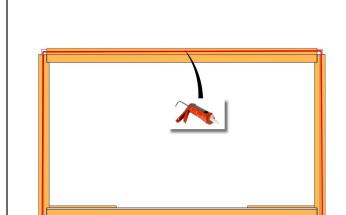
Apply a continuous 3/8" bead of sealant along the backside of the nailing flange. Bead must run around both sides and across the head, in line with and completely covering the nail holes.
