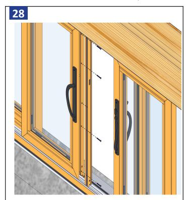
Install astragal to one active panel with provided screws. Make sure the lock notch matches up with lock.
