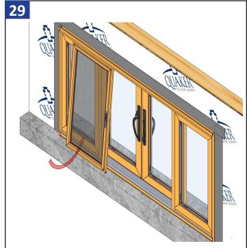
Angle the screen panel with the top inserted into the head track, and then lift and set the bottom rollers on the roller track. Adjust rollers as needed to insure the panel is level, square, and slides smoothly. Repeat above steps for the other screen.
