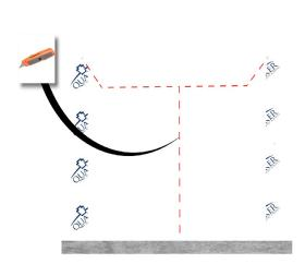
Apply the house wrap according to the manufacturer's instructions and cut T-pattern opening as shown above. Cut top flap angles at 45 degrees and 1" longer than the width of flashing tape being used.
