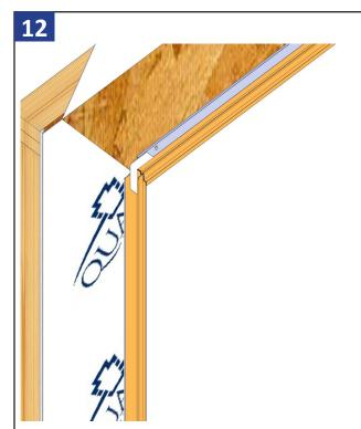
Temporarily tack the door into place using 2" galvanized roofing nails through the pre-punched hole on one top corner of nailing flange.
