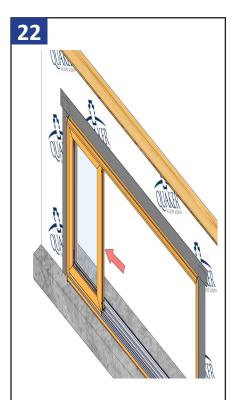
Slide the panel tight against the frame keeping the panel flush with the fixed panel extrusion in the sill.
