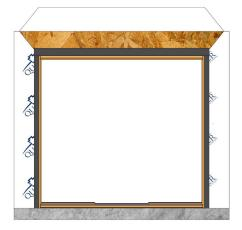
Apply a 3/8" sealant bead to the top exterior edge of door frame before installing the drip cap.
