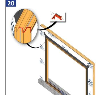
Seal the inside edge corners at the head and sill where the fixed panel will set in the frame.
