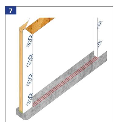
Apply three 3/8" continuous beads of silicone across the entire width of the rough opening sill, and a 3/8" continuous bead of silicone %" from each side of the rough opening as shown above.
