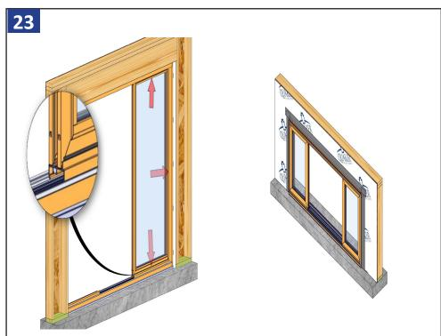
Install wedge gasket in the sill, head, and jamb around the interior of the frame and panel to secure the panel in place.
