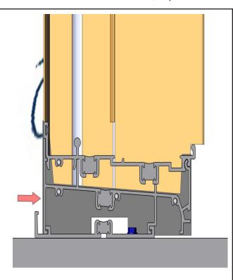
Center and set the door frame into the rough opening, making sure there are equal gaps on both sides of the door.
