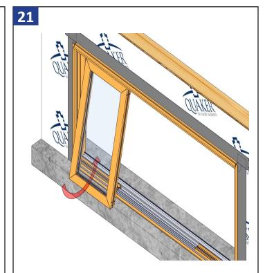
Angle the fixed panel with the top inserted into the head track, and then lift and set the bottom of the panel on the fixed panel extrusion in the sill.
