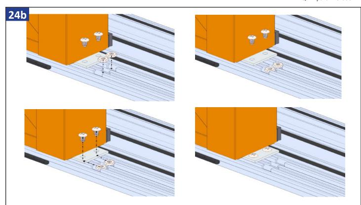
For ModernVu and M204 units, install the meeting rail using supplied (MH8-18X1/2 TK2) screws in the head, and (MP10/24X3/8 & 10-24 NUT) screws and nuts in the sill angle brackets.
