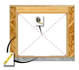
Check that the door is square. Adjust shims as needed until diagonal measurements are within 1/8". Level at the sill and plumb the frame.
