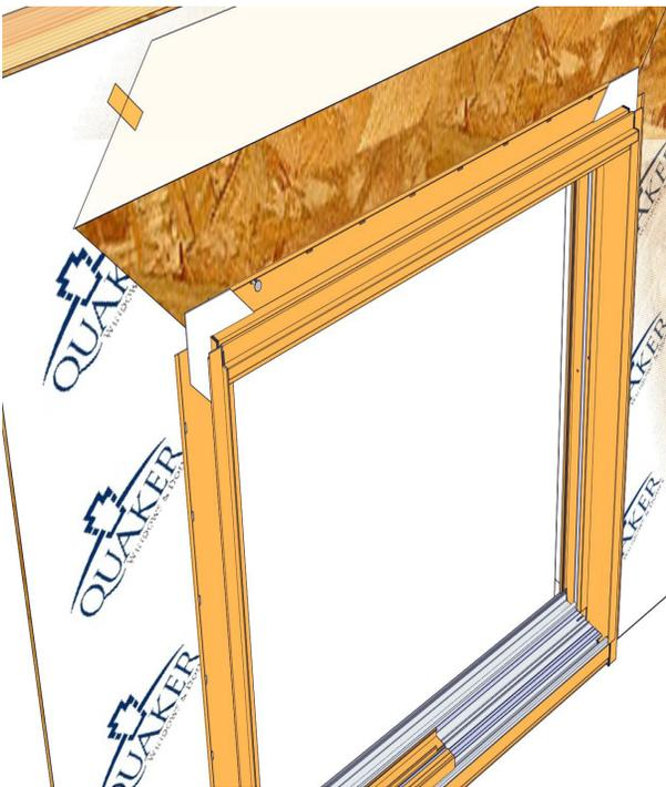
Temporarily track the door into place using 2" galvanized roofing nails through the pre-punched holes on one top corner of the nailing flange.
