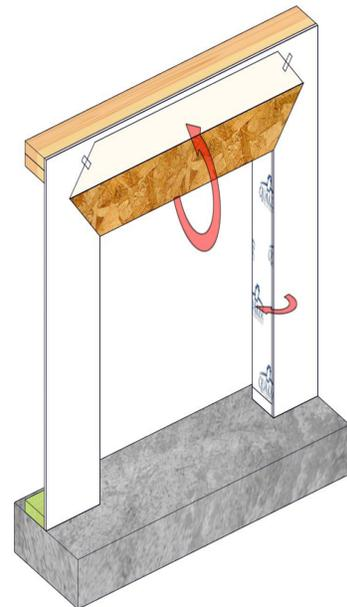
Fold the house wrap to the interior and staple it to the interior framing. Fold the house wrap flap up and temporarily tape it in place.
