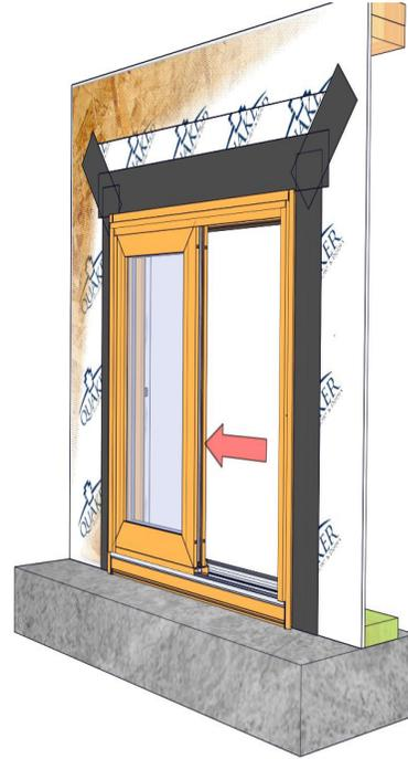
Slide the panel tight against the frame keeping the panel flush with the fixed panel extrusion in the sill.
