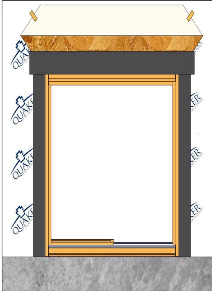
Apply a 3/8" sealant bead to the top exterior edge of door frame before installing the drip cap.
