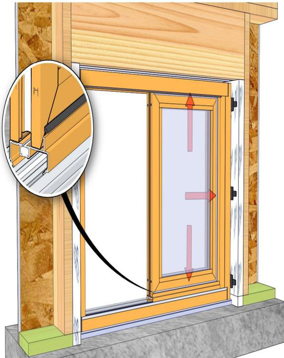
Install wedge gaskets in the sill, head, and jamb around the interior of the frame and panel to secure the panel in place.
