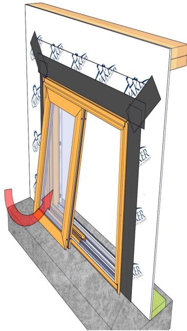
Angle the fixed panel with the top inserted into the head track, and then lift and set the bottom of the panel on the fixed panel extrusion in the sill.
