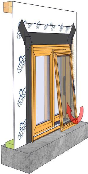
Angle the screen panel with the top inserted into the head track, and then lift and set the bottom rollers on the roller track. Adjust rollers as needed to insure the panel is level, square, and slides smoothly.
