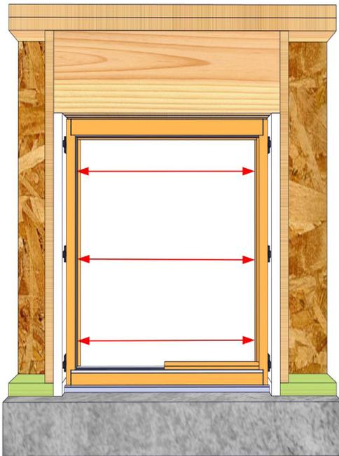
Check that the door frame is not bowed. Adjust shims as needed until measurements are within 1/8". Finish fastening the unit every hole or a minimum of 12" on center.
