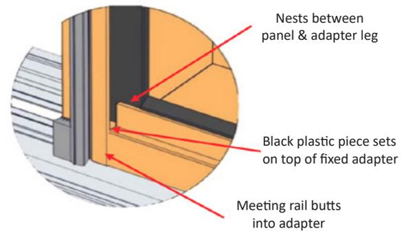
Apply a bead of sealant to inside edges of meeting rail before sliding the pre-assembled meeting rail against the fixed panel.
