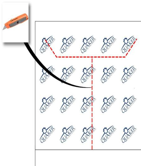
Apply the house wrap according to the manufacturer's instructions and cut T-pattern opening as shown. Cut top flap angles at 45 degrees and 1" longer than the width of flashing tape being used.
