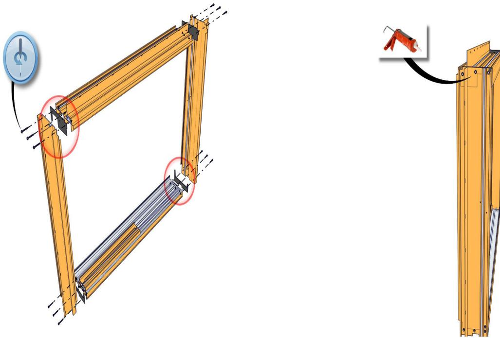
Assemble jamba to head and sill assembly with the 12 fasteners provided (MH8-18X11/2 LP). Make sure to use the two head and sill gaskets provided, and seal around all screw heads and outside corners.
