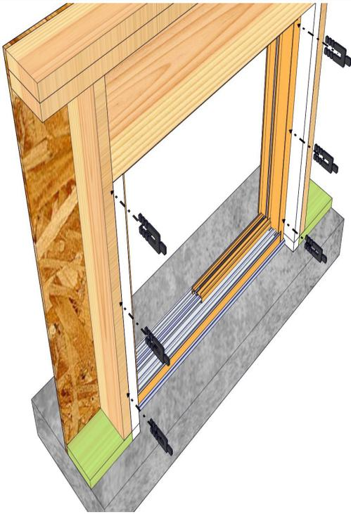
Shim at the sides of the door, and at the lock location as shown above. Never shim at the head.
