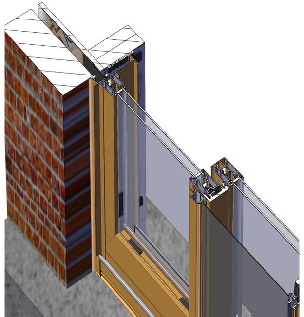
Apply sealant continuously around entire perimeter of opening, filling interior 1/3 of cavity using low expanding foam or backer rod and sealant.
