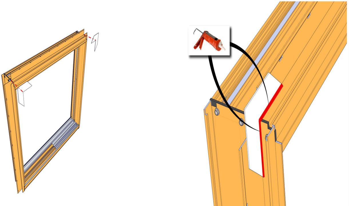
Clean the nail fin corners prior to installing the corner gaskets to the exterior side of nail fin corner gaps. Apply sealant along the edge where the gasket meets the window frame.
