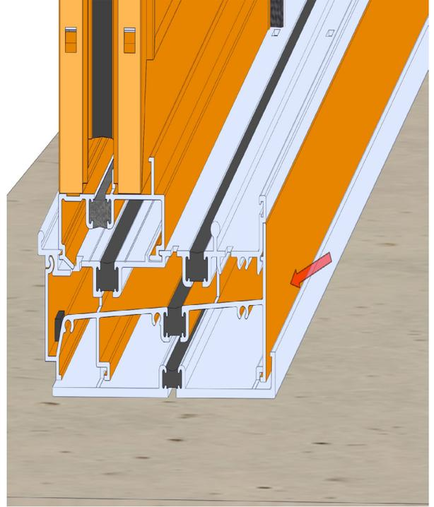
Center and set the door frame into the rough opening, making sure there are equal gaps on both sides of the door. Angle the door frame with the top tilted out, and set the exterior sill frame inside the exterior leg of the sub-sill anchor plate as shown above. Push the frame in against the framing to lock the sill into the sub-sill anchor plate.
