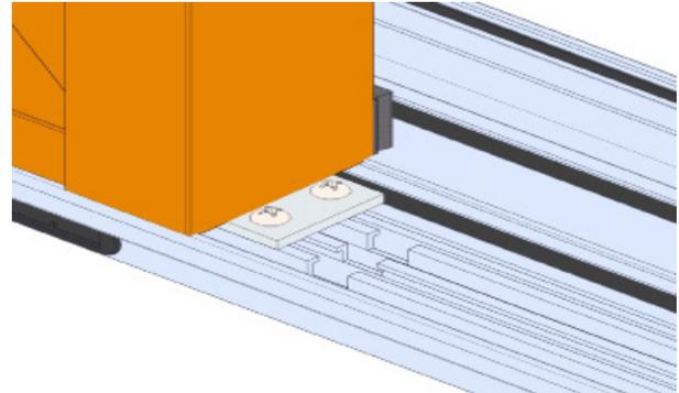
Install the meeting rail using supplied (MH8-18X1/2 TK2) screws in the header, and (MP10/24X3/8 & 10-24 NUT) screws and nuts in the sill angle brackets.
