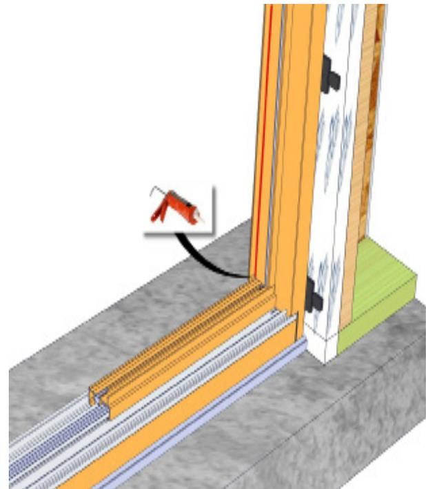
Seal the inside edge corners at the head, sill, and jamb where the fixed panel will set in the frame.
