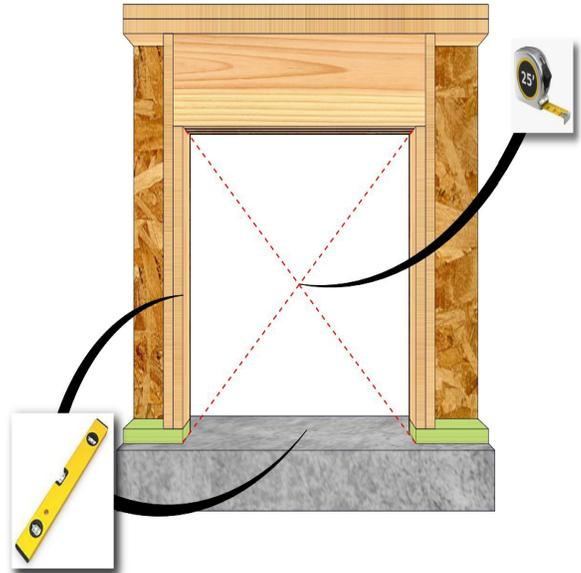
Check that the opening is square. The diagonal measurements need to be within 1/8" of each other. Verify the rough opening is plumb and level. The sill plate beneath the unit must be level for proper unit operation.
