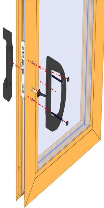
Install handle set using provided instruction found in the hardware box using the 1 7/8" door thickness section.
