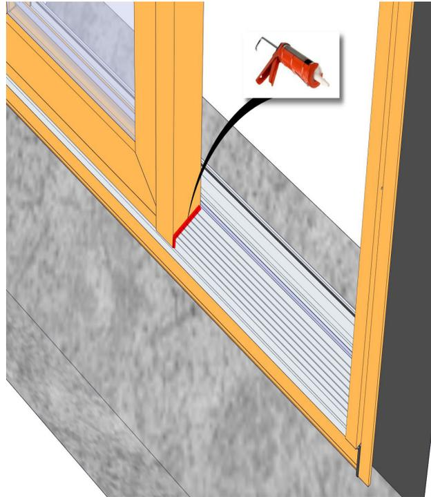
Install threshold on the exterior side of frame covering the bottom angle brackets. Seal around the two ends of the threshold against the frame as shown above.
