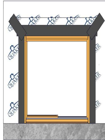
Unfold the house wrap top flap and tape the angled seams as shown.
