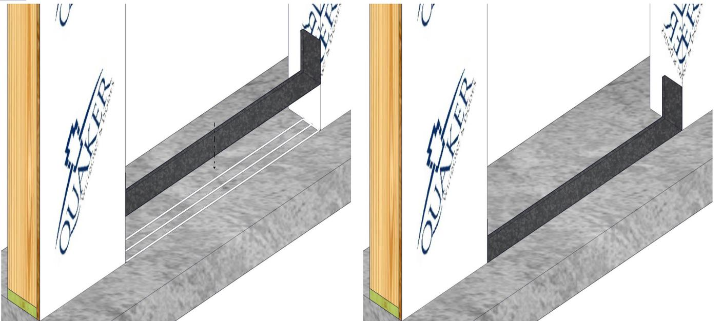
Install a sill pan flashing with minimum 1/2" interior leg (**by others**). If installing the door with the position fin set the sill pan 3 3/16" in from the exterior.
