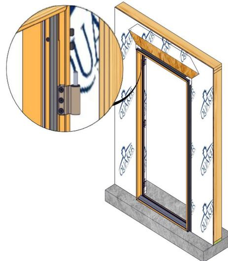
Install and fasten the door unit in place using fasteners by others per anchorage calculations. Typically, a #12 screw 6" from the top and bottom and 16" on center thereafter. Always follow the anchorage calculations and fastener/anchor manufacture's guidelines for proper edge distance, load capacity and installation techniques.
