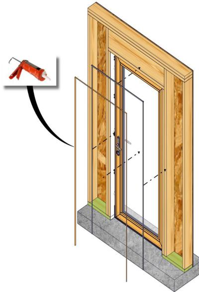
Apply insulation and a continuous bead of sealant around the entire interior perimeter of the door unit.
