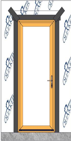
Flip down upper flap of WRB so it lays flat across head flashing, then trim 1" - 2" above the door opening. Tape along all cuts in WRB and across head of the door with flashing tape.
