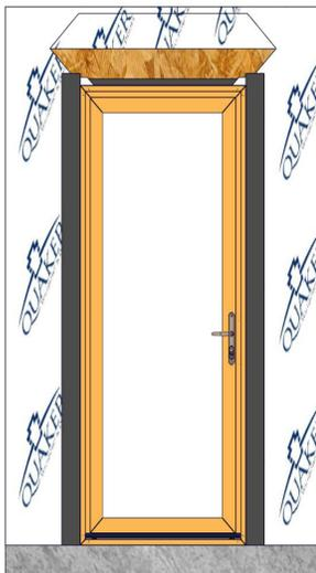
Cut two pieces of flashing tape for jamb flashing extending 1" above head position fin. Remove release paper and press tightly along sides of door frame.
