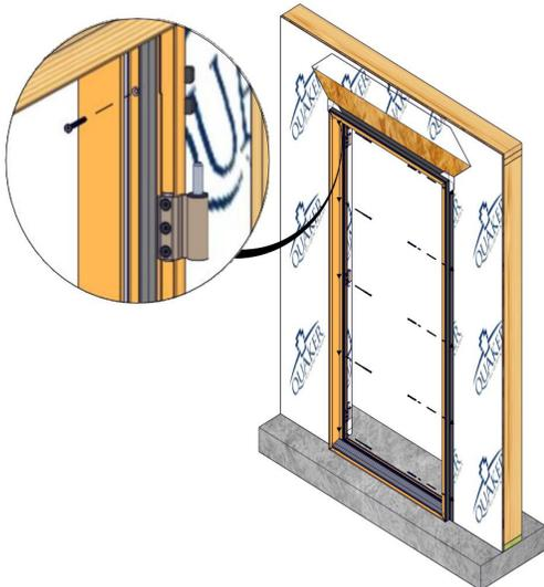
Drill a countersink hole through the jambs in the exterior track per anchorage calculations. **Quaker Window Products does not supply or claim liability for anchorage/fastener calculations. It is the installer/client's responsibility for structural adequacy of the anchorage and fasteners.** Typically, a #12 screw 6" from the top and bottom and 16" on center thereafter.
