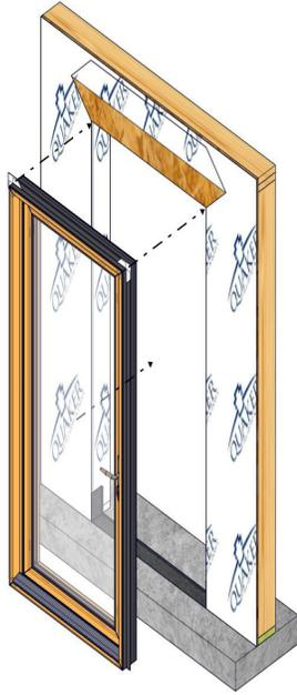
Center and set the door frame into the rough openings pushing the position fin tight against exterior framing. **Note: DO NOT nail or fasten through the position fin.** Level at the sill and plumb the frame. Shim under the frame to bring to level in necessary.
