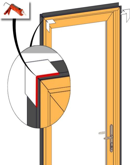
Install the two top foam corner key gaskets over the exterior side of the position fin corner gaps. Seal the exterior corners where the foam gasket meets the position fin.
