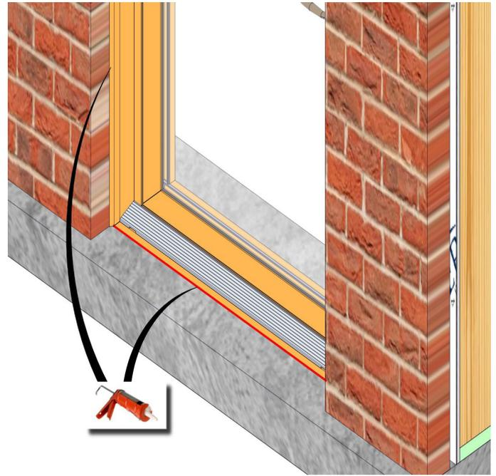
Apply a continuous bead of sealant across the full length of the sill and around exterior perimeter of door unit.
