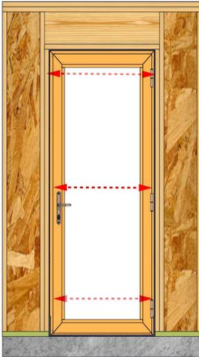
Verify the door is square, level, and plumb. Check the spacing around the door at the top, middle, and bottom to make sure the door is not over shimmed. See hinge and lock adjustment guides if adjustments are needed.
