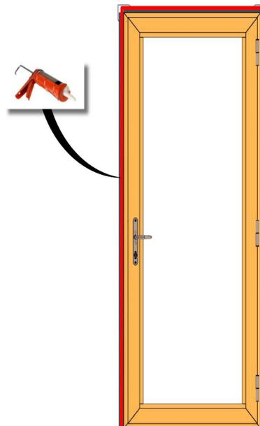
Install a continuous bead of sealant around the interior side of the position fin.
