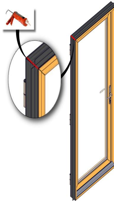
Snap the fin into place with short side of the flange facing the exterior. Seal the corners of the position fin.
