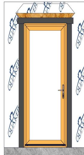
Cut a piece of flashing tape for the head flashing, which extends beyond outer edges of jamb flashings. Remove release paper and install completely covering position fin and adhering to exposed sheathing or framing members.
