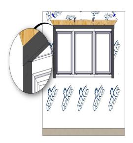
Apply flashing over the top head board and against the sheating, overlapping the side flashing as shown. Smooth using a J-roller. Side flashing cannot extend above the top flashing. Doing so could result in product or property damage.
