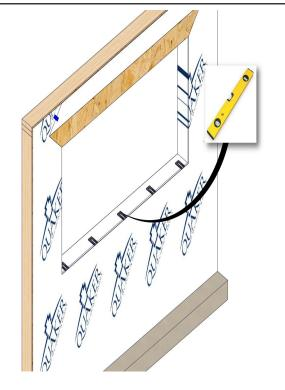
Verify the rough opening is plumb and level. The sill plate beneath the unit must be level for proper unit operation.
