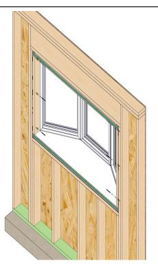
Check that the frame is plumb and level. Adjust shims as needed. Install fasteners through the side jambs into framing starting 2" from the corners and 16" on center there after.
