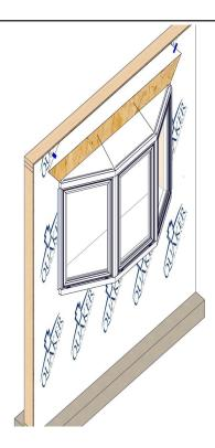
Temporarily fasten with a single fastener at the top of the jamb nail flanges.
