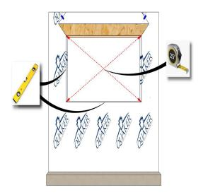
Measure and verify the opening is sized correctly. The rough opening should be a minimum 1/2" (but not to exceed 1") wider and taller than the unit. Allow additional space for flashing thickness, installation clips, joining components, and their fasteners.
