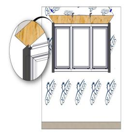
Apply flashing tape at the sides of the window, overlapping sill flashing as shown. Smooth using a J-roller. Extend tape a minimum of 2" pass window frame.
