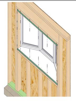
Install fasteners across the seat board and head.
