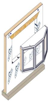
Center the window in the opening, setting the window on the shims. Make sure shims are positioned under each side jamb and the unit is flush with the interior wall surface. 5
