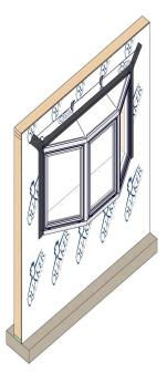
Apply sealant continuously around the entire perimeter of opening, filling interior 1/3 of cavity using low expanding foam or backer rod and sealant.
