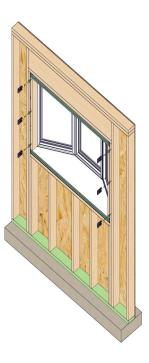
Shim at the sides of the window, and at the check rail locations. Never shim at the head.
