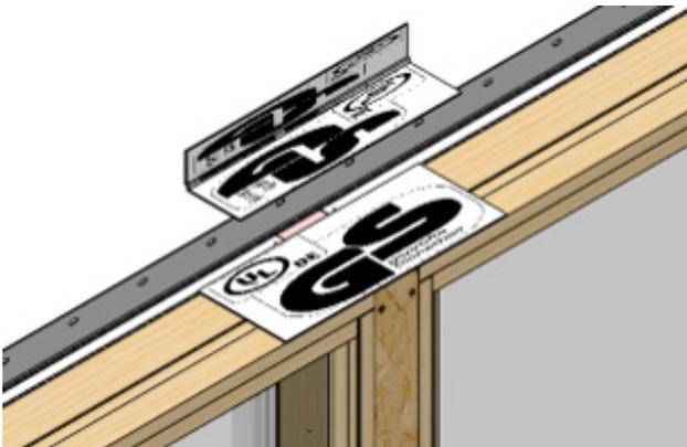
Install one 4" flashing tape flush with interior face of window over the head mull gap.
