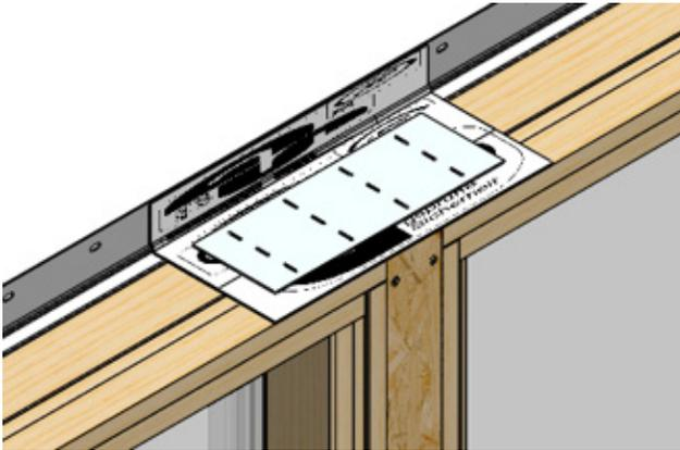
Install mending plate centered over mull gap and staple or screw into place. (Do not use fasteners longer than  $\frac{3}{4}$ " )
