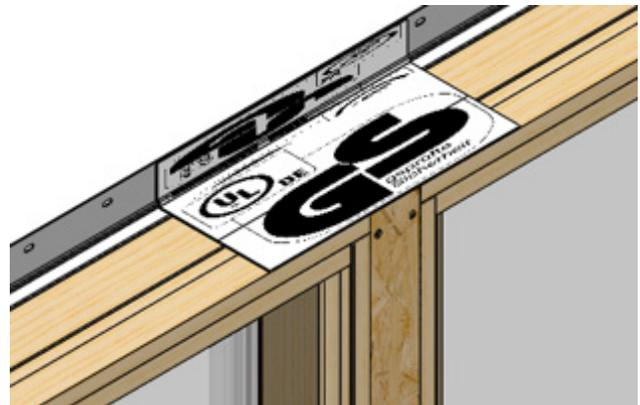
Install another 4" flashing tape over lapping the other flashing tape and up the backside of nail fin.
