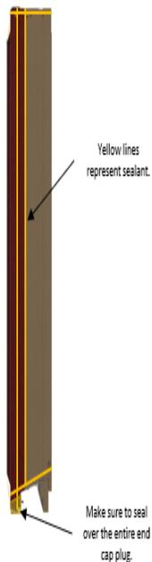
Place two continuous beads of silicone down the entire side of one window to be mulled. Place another bead of silicone at the head and sill of mullion jamb the full width of fame as shown above.
