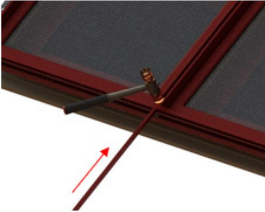
Cut the C-mull keys to the length of the unit (width or height) to be mulled.
