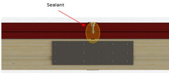
Seal both ends of the mull gap with silicone.
