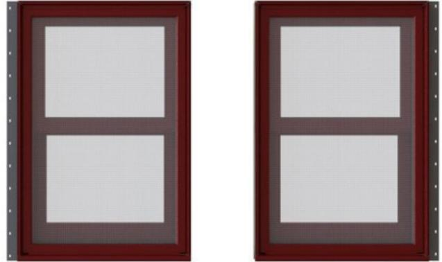
Remove the nailing fin from each unit where the mull will connect them, as well as the head and sill fins if horizontal mulling. Remove fins by pulling them out of slot and dispose of properly. Head and sill fins will be replaced with full length pieces.
