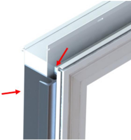
Apply the mullion to the side of the window aligning the mullion with the j-channel pocket. Make sure the mullion doesn't stick past the j-channel pocket. Press firmly to engage the double-sided tape.
