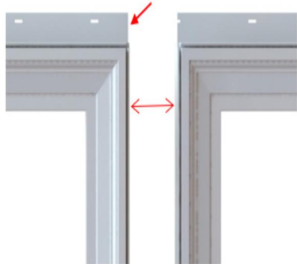
Using a utility knife score and remove all of the nailing fin from each unit where the mull will connect them. Make sure to cut the head and sill nail fins back flush with ripped nail fin.
