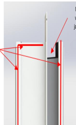
Make sure any excess weld is cleaned so the jamb filler will set flush
