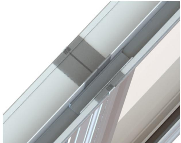
Apply sealant to the bottom edge of the jamb filler before installing it in the j-channel pocket at both ends of mullion, and add sealant to gap between filler and mull key.
