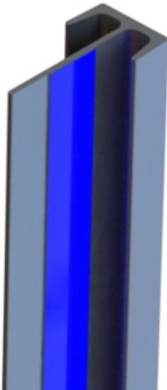
Cut the T-reinforcement mull 2" less than window unit. Clean mull with alcohol to remove any oil. Apply a strip of double-sided tape to one side of mull as shown above.
