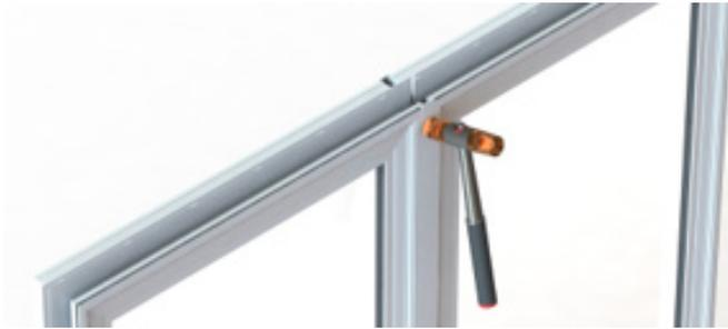
Install the mull key flush with one side of unit and hammer into place with rubber hammer.
