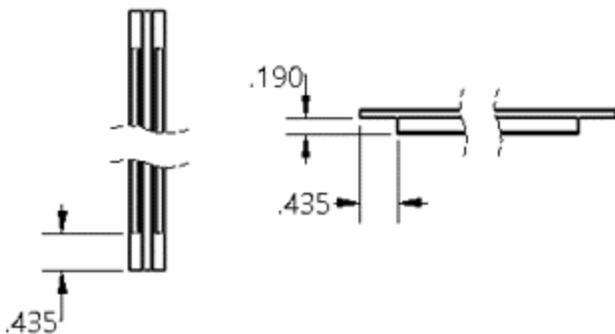
Cut the C-mull keys to the length of the unit (width or height) to be mullied. Notch both ends of mull key with a utility knife or chisel per dimension shown above.
