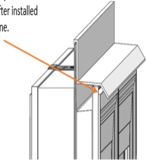
Install drip cap over the nail fin the full length of mull units at the head.
