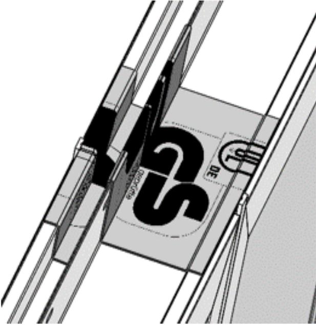
Apply self-adhesive flashing tape over the top side of mull gap and over nail fin.
