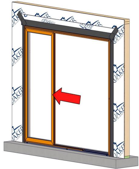
Slide the panel tight against the frame keeping the panel flush with the fixed panel extrusion in the sill.
