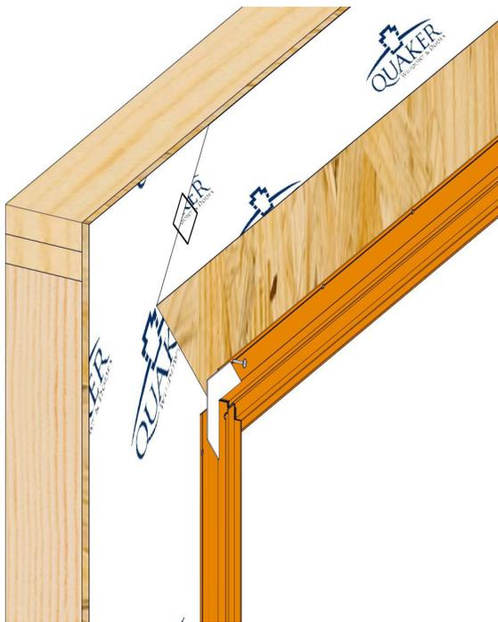
Temporarily tack the door into place using 2" galvanized roofing nails through the pre-punched hole on one top corner of nailing flange.
