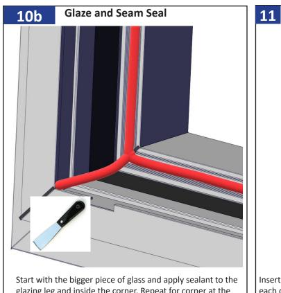
glazing leg and inside the corner. Repeat for corner at the head.
