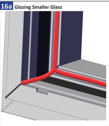
Move to the smaller piece of glass and apply sealant to the glazing leg and inside the corner. Repeat for corner at the head.
