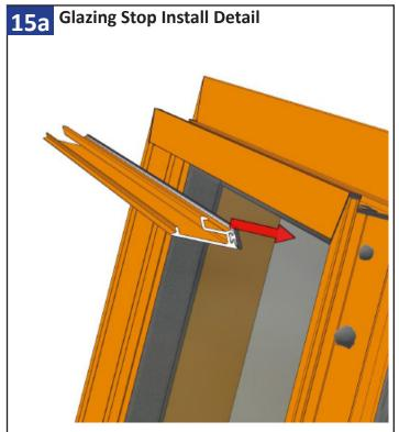
Install the stop by rolling the stop into place. A mallet may be required to persuade the stops to lock into place. Repeat for remaining glazing stops.
