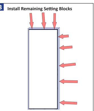
With the glass in the frame, install the remaining setting blocks around the glass perimeter. Place a block no more than 6 inches from each corner, and along the perimeter of the glass every 18 inches.
