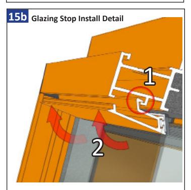
Install the stop by rolling the stop into place. A mallet may be required to persuade the stops to lock into place. Repeat for remaining glazing stops.
