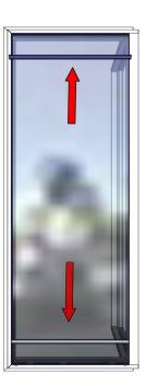
Install the horizontal glazing stops first at the head and sill. Then install the the 1 vertical stop.
