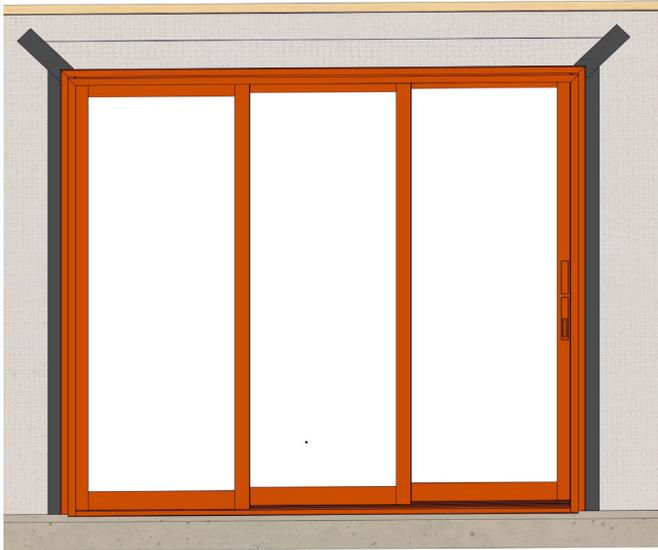
Unfold the house wrap top flap and tape the angled seams as shown.
