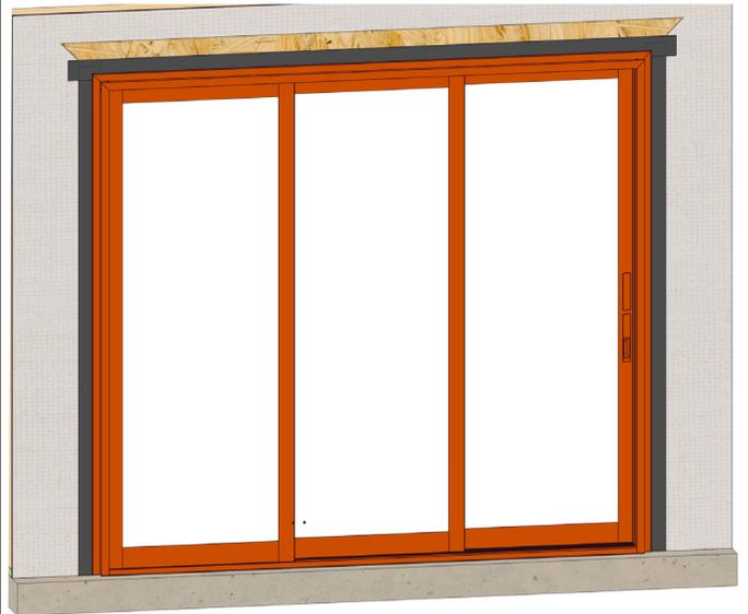
Apply a 3/8" sealant bead to the perimeter edge of door frame before installing the drip cap. Apply flashing tape over the drip cap leg, overlapping the side flashing as shown. Smooth using a J-roller.
