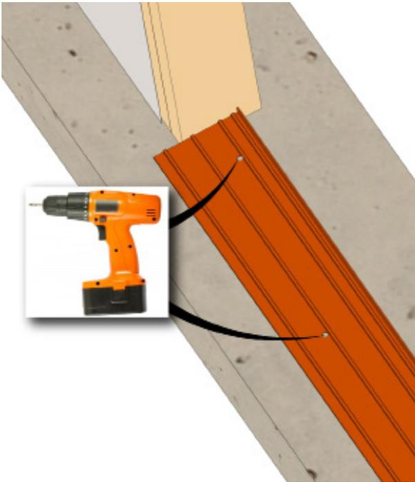
Locate second and third leg and drill holes directly behind them. Drill holes through the sill pan, 3" from each end and then 14" on center for the length of the pan, alternating between the 2 tracks.
