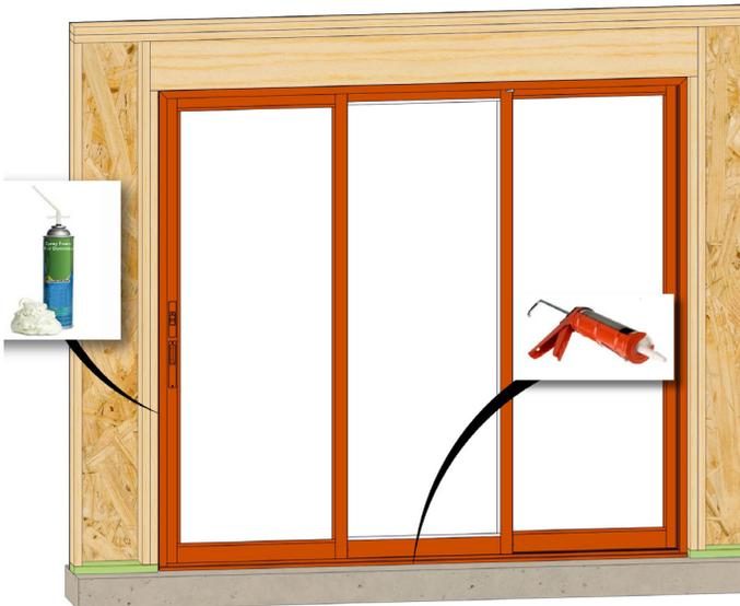
Insulate the gap between the door and framing with minimally expanding spray foam, and seal the entire interior perimeter with sealant.
