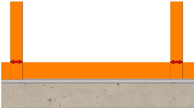
Lock the active panel, and adjust rollers on all panels so they roll smoothly. Start with the active panel and work your way towards the fixed panel. Check the reveal of the glass at the bottom of panels and adjust as needed to line up all panels.
