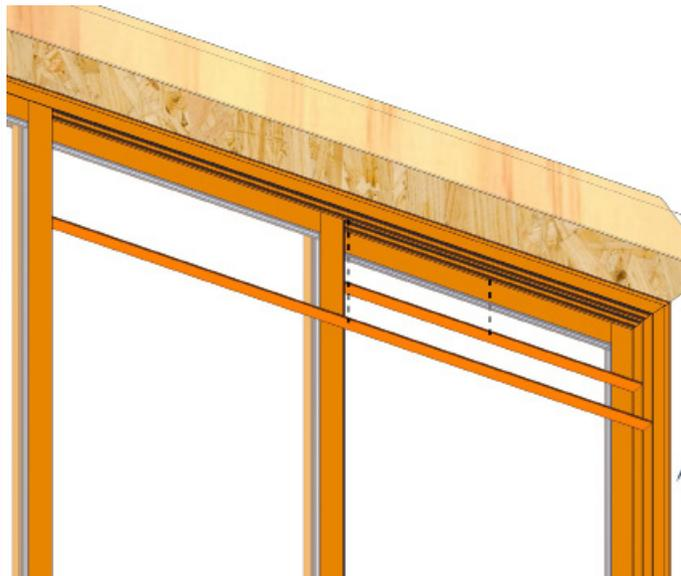
Next install the short and long header covers in the exterior and middle tracks. Trim covers to fit if needed.
