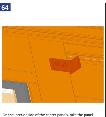
pickups (Part #: M25296-PCS) and #10 screw (Part #:MF10AX1)that is provided. Take screws and attach the pickups. Install the panel pickup where the holes are already fab'd on the interior side of the door.
