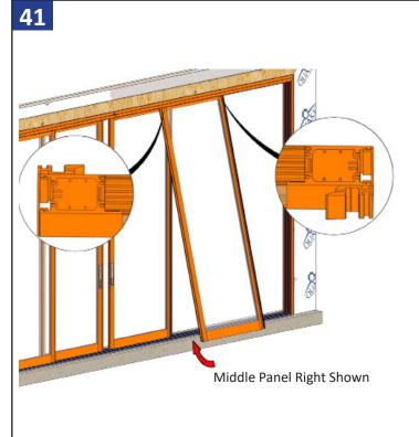
Repeat for the middle panel on the right placing it in the center tracks. Make sure the panel overlaps the center panel on the right so the interlocks will engage properly.
