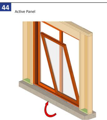
On the interior side set the active panel on the roller track. Make sure the panels are overlapped when installing so the interlocks will engage properly. Slide panel to the fixed jamb. Make sure the closure captures active panel.
