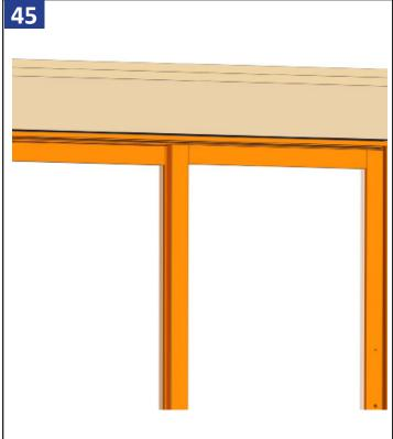
Take the head closure, trim to fit between the jamb closures, and slide it over the head of the panel.
