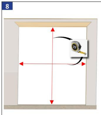
Measure and verify the rough opening is sized correctly. The frame opening should be 13/16" wider and 1/2" taller than the framed unit. Allow additional space for flashing thickness, installation clips, joining components, and their fasteners.
