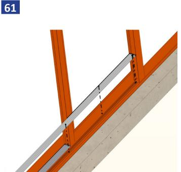
Next install the exterior sill cover. DO NOT HIT THE SILL COVERS DIRECTLY DURING INSTALL!
