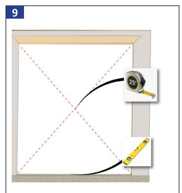
Check that the opening is square. The diagonal measurements need to be within 1/8" of each other. Verify the rough opening is plumb and level.
