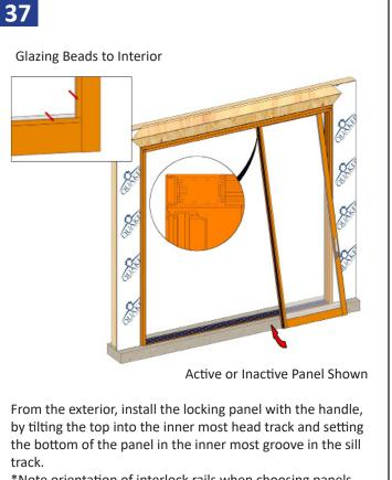
\*Note orientation of interlock rails when choosing panels. \*Note glazing beads are to the interior side.
