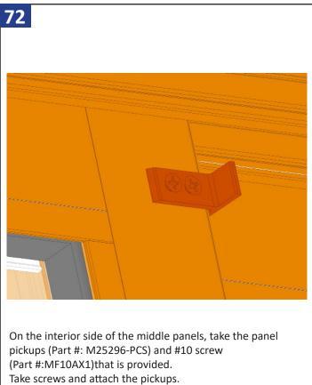
Install the panel pickup where the holes are already fab'd on the interior side of the door.
