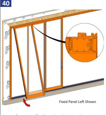
Repeat for exterior (fixed) panel, setting it into the exterior tracks in the head and sill. Make sure the panels are overlapped when installing so the interlocks will engage properly.
