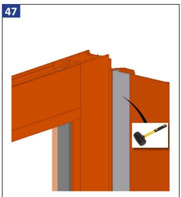
Next install the pocket closure cover with a rubber mallet. Be care not to dent the cover or closure.
