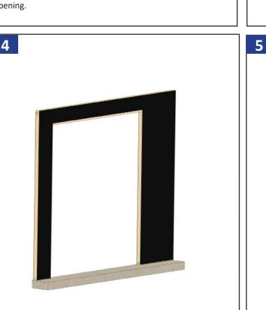
Prior to starting, line inside of the exterior wall with black board.
