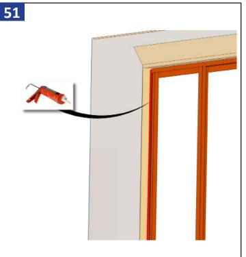
Apply a 3/8" bead of sealant under where the extieror closure will be installed. Closure will run from head to sill. Install the closure.
