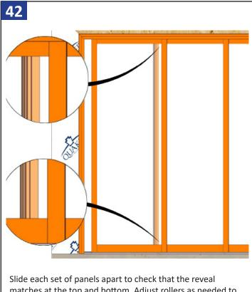
Slide each set of panels apart to check that the reveal matches at the top and bottom. Adjust rollers as needed to match reveal across panels.
