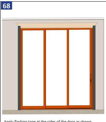
Apply flashing tape at the sides of the door as shown. Smooth using a J-roller. Extend tape a minimum of 2" past door frame, but not more than the thickness of the flashing tape.
