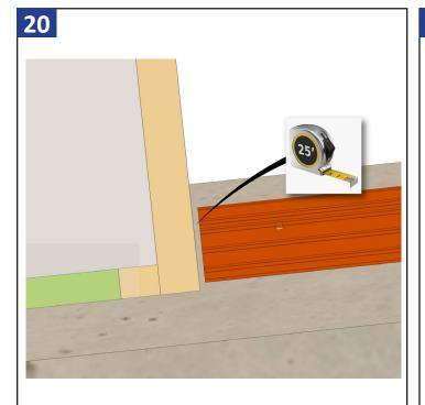
Allow a 1/4" gap between the rough opening and the sill pan. This should also include a 1/4" from the back of the tank.
