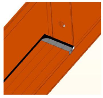
Take the sill covers and cut the end of the cover that doesn't have the molded part on the end.
