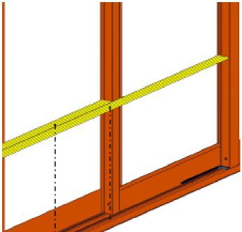
Lay out sill cover before installing, start with the sill cover closer to the interior.
