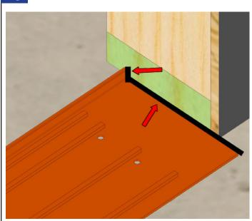
Set the sill pan in place along the wall and upturned leg apply silicone. Be sure to tool in the sealant.
