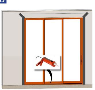
Check to ensure a continuous bead of sealant at the exterior base of the sill. Be sure to not block the weeps on the bottom of the sill.
