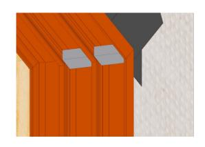
Place 1 dust plug in each track where the heads meet, as shown in the picture above, except the locking panels.
