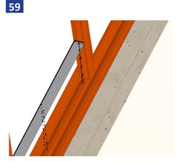
Install the interior sill cover. DO NOT HIT THE SILL COVERS DIRECTLY DURING INSTALL!
