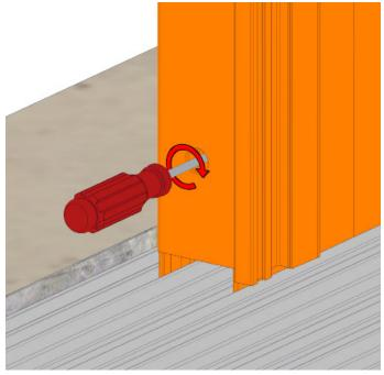
Use a #2 phillips screwdriver to engage the roller adjustment on both sides of a panel. Turn clockwise to raise the panel and provide smooth rolling. If possible, lift the panels slightly when adjusting to take pressure off the rollers. Roll panel back and forth 2-3 times to verify roller height is set. Repeat this step for each panel installed.
