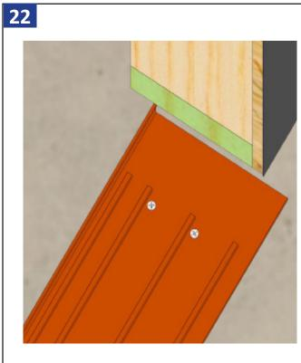
Using a screw with the head is shorter (less than .150"), screw down the sill pan.
