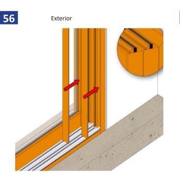
On the exterior jambs of the door, install two frame jamb covers - one in the middle track and one in the outermost track. Trim to fit. If a mallet is needed to install the jamb covers, use a wood block in between. DO NOT HIT THE JAMB COVERS DIRECTLY!
