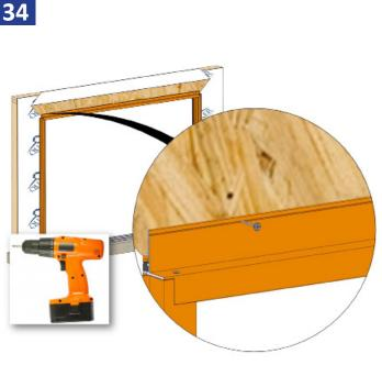
Fully fasten the screws down now to hold the frame in place.
