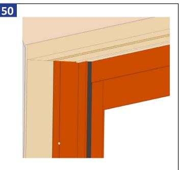
Take the exterior closure interlock (Part #: M25389) and cut it to length. Lock the door system. Rough fit it in the opening, and shim if necessary. If unable to lock, the closure needs to be shimmed out toward the lock.
