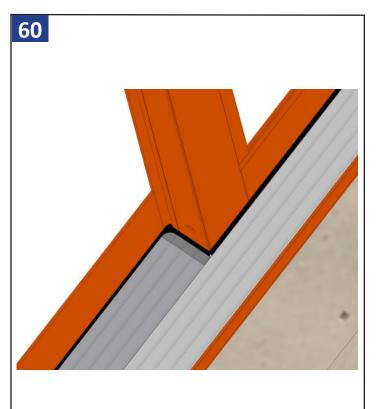
On the exterior sill cover, cut away the weather strip where it meets the sill cap you just previously installed. NOTE: ON FIXED PANEL MEASURE FROM PANEL TO FRAME AND SUBTRACT 1/16", CUT, THEN PLACE AGAINST FRAME.
