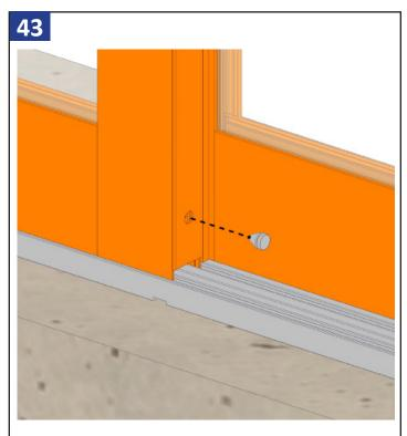
Once all panels have been adjusted install the panel bumpers (Part #: 9309K86) into each roller adjustment hole.
