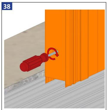
Use a #2 phillips screwdriver to engage the roller adjustment on both sides of a panel. Turn clockwise to raise the panel and provide smooth rolling. If possible, lift the panels slightly when adjusting to take pressure off the rollers. Roll panel back and forth 2-3 times to verify roller height is set. Repeat this step for each panel installed.
