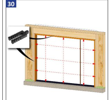
Check that the door frame is not bowed at jambs or head, a string line may be required. Adjust shims as needed but verify measurements are within 1/16".
