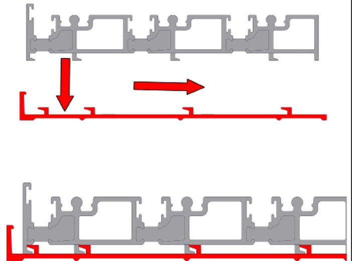
Push the sill down and then toward the exterior to lock in the sill to the sill pan.
