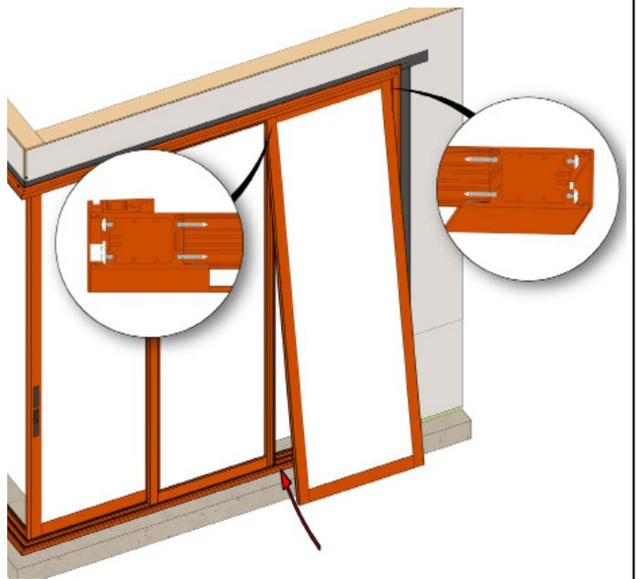
Repeat for exterior panel, setting it into the exterior tracks in the head and sill. Make sure the panels are overlapped when installing so the interlocks will engage properly.
