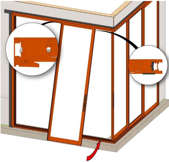
From the exterior, install the locking panel with the handle, by tilting the top into the inner most head track and setting the bottom of the panel in the inner most groove in the sill track.
