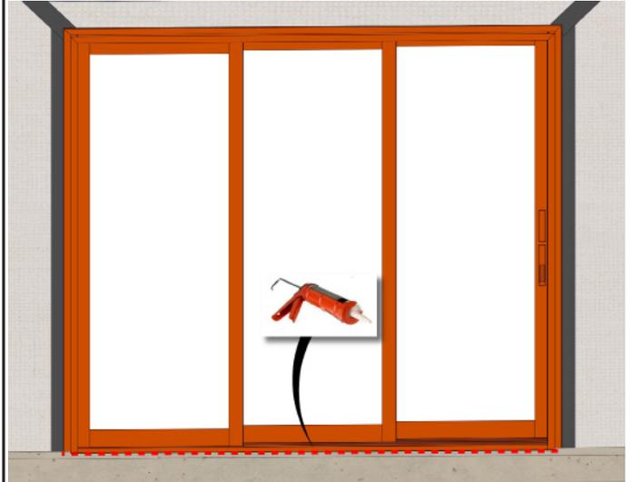
Apply a continuous bead of sealant at the exterior base of the sill. Be sure to not block the weeps on the bottom of the sill.
