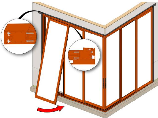
Repeat for exterior panel, setting it into the exterior tracks in the head and sill. Make sure the panels are overlapped when installing so the interlocks will engage properly.
