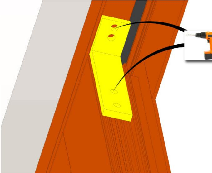
Take the **Fixed Panel Bracket**, slide it to the head drill holes for the tri-wing screws.
