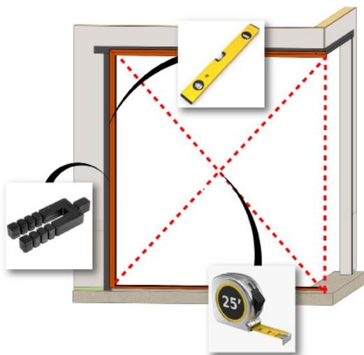
Check that the door frame is not bowed at jambs or head, a string line may be required. The jamb cover can be used to ensure equal spacing between the sill and head. Adjust shims as needed but verify measurements are within 1/16". Repeat for the other side.
