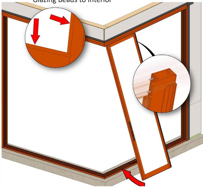
From the exterior, install the locking panel with the handle, by tilting the top into the inner most head track and setting the bottom of the panel in the inner most groove in the sill track.
