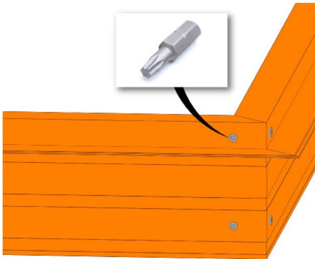
Start 4 screws (Part #: FE FAST2) into the keys at the mitered corner.
