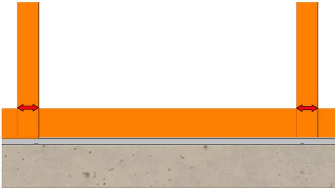
Lock the 2 middle panels together, and adjust rollers on all panels so they roll smoothly. Start with the 2 hardware panels and work your way towards the fixed panels. Check the reveal of the glass at the bottom of panels and adjust as needed to line up all panels.
