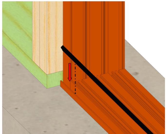
Locate the interior side of the sill. Push the sill down and towards the exterior to lock in place. Take the wedge gasket (Part #: 4874-02-00) and press in place. Note: This will run the whole length of the sill pan.
