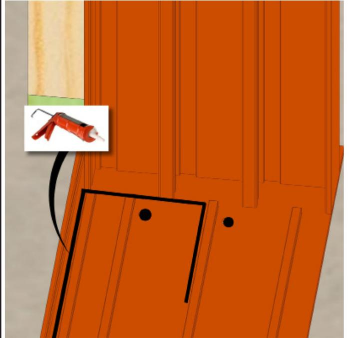
Run a bead of silicone along the wall, up the leg of the flashing pan, and along the interior most lip.
