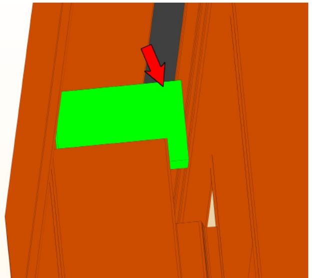
Slide the fix panel fully into the frame jamb, then take the frame head dust plug and remove backing. Slide the dust plug in between the head and the top of the fixed panel. The edge of the panel and the face of the dust plug should be flush. Repeat this step on the other side.
