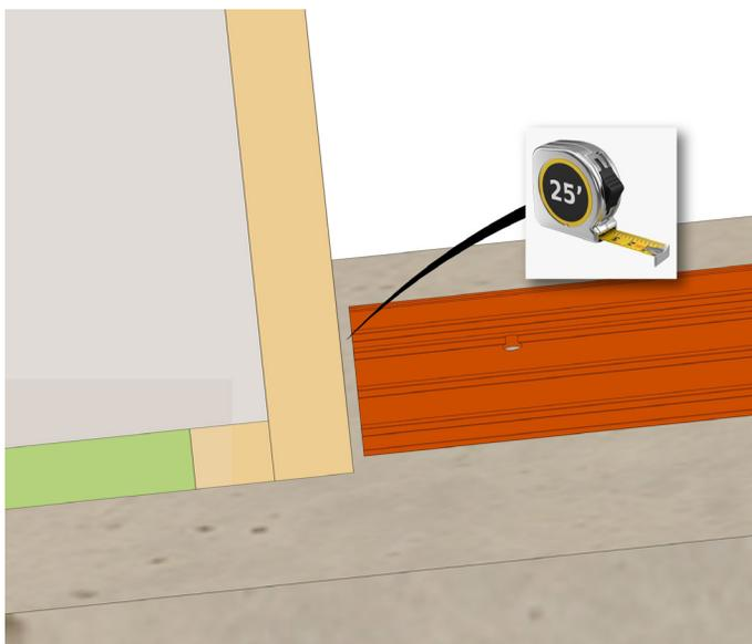
Allow a 1/4" gap between the rough opening and the sill pan.
