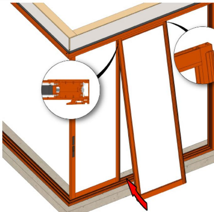
On the exterior side repeat for the middle panel, setting it into the middle tracks in the head and sill. Make sure the panels are overlapped when installing so the interlocks will engage properly.
