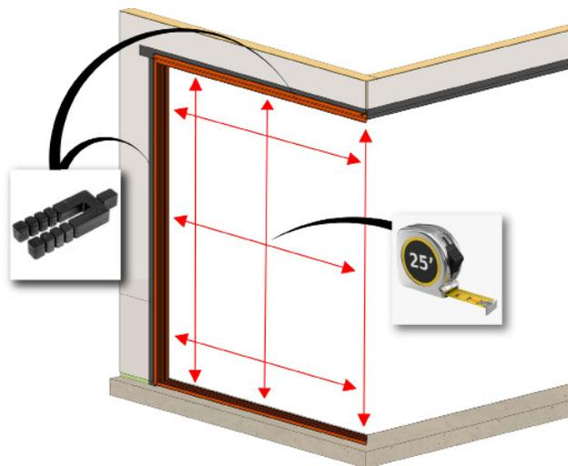
Check that the door frame is not bowed at jambs or head; a string line may be required. The jamb cover can be used to ensure equal spacing between the sill and head. Adjust shims as needed, but verify measurements are within 1/16".
