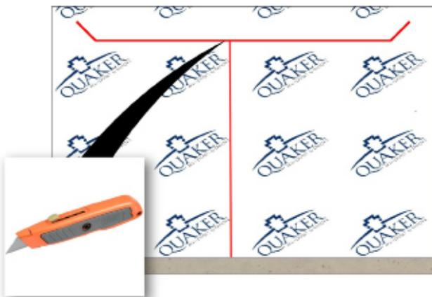
Apply the house wrap according to the manufacturer's instructions and cut T-pattern opening as shown above. Cut top flap angles at 45 degrees and 1" longer than the width of flashing tape being used.
