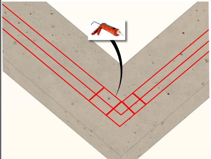
On each side of the 90 degree corner apply 2, 3/8" beads of silicone across the 3 beads of silicone as shown above.
