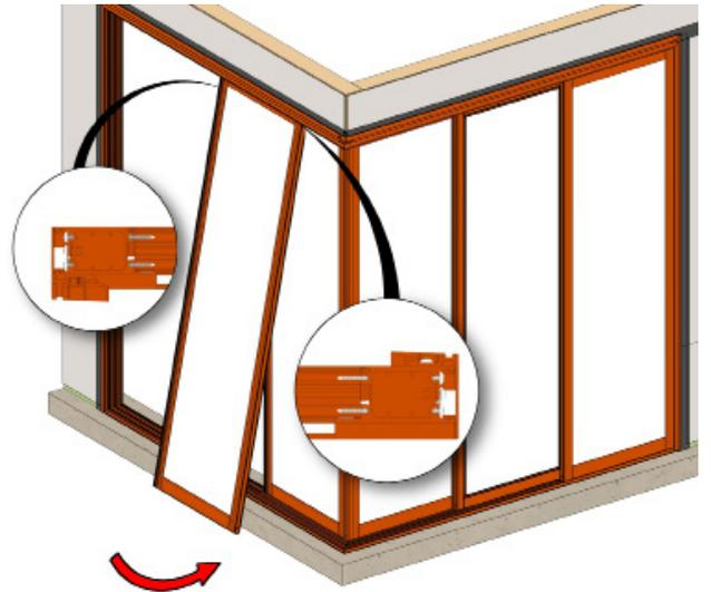
On the exterior side repeat for the middle panel, setting it into the middle tracks in the head and sill. Make sure the panels are overlapped when installing so the interlocks will engage properly.
