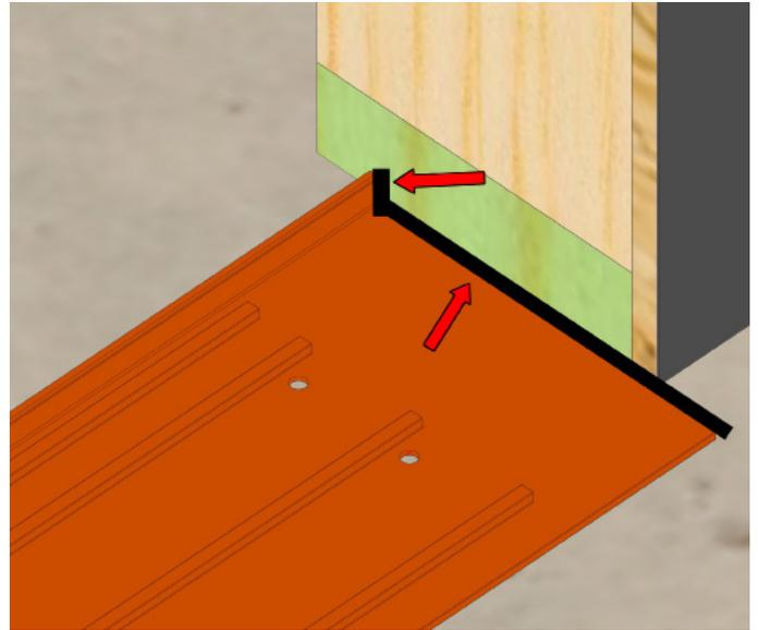
Silicone along the wall and upturned leg. Be sure to tool in the sealant.
