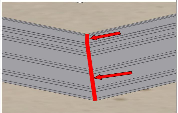
Apply silicone where the 2 sill pans meet, up the interior most leg, and makes a 90 degree corner. Make sure this joint is tight.
