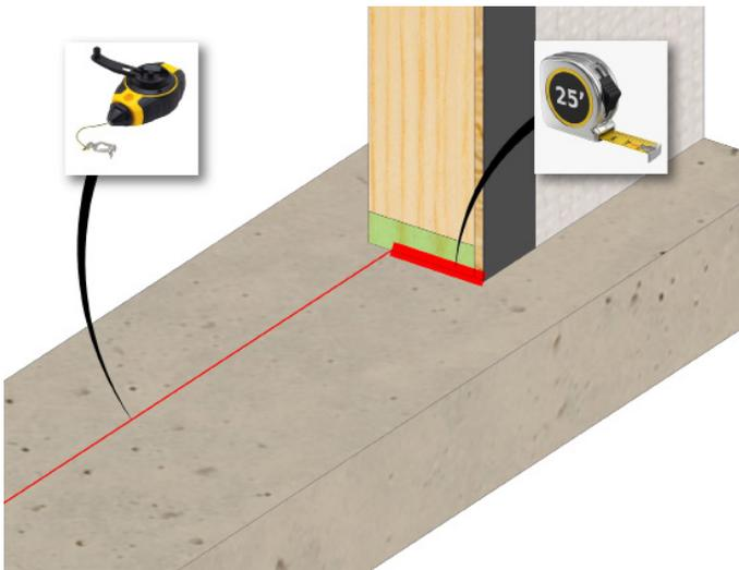
Measure and set a chalk line on the sub floor 4 7/8" in from the exterior wall face. Dry fit the provided sill pan system with the rear upturned leg on this line.
