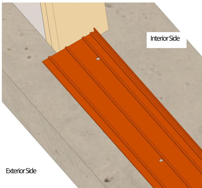
Rough fit the sill pan in place to ensure of proper fitment.
