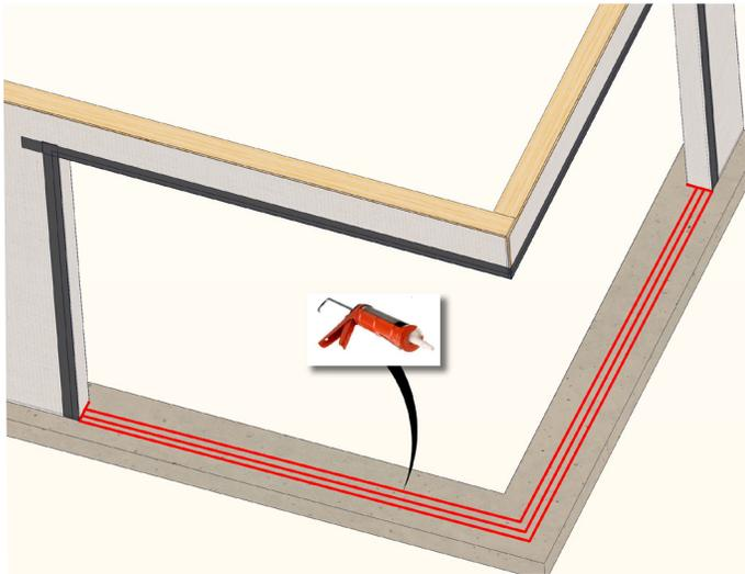
Apply three 3/8" continuous beads of sealant across the entire width of the rough opening sill where the sill pan will sit. Be sure to make a continuous path around the corner as shown above. Apply two 3/8" continuous beads of sealant the width of the pan, 1/2" from each side of opening as shown above.
