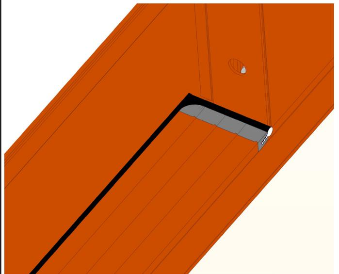
Take the sill covers, and cut the end of the cover that doesn't have the molded part on the end. (Molded part is shown in the picture above in gray.)
