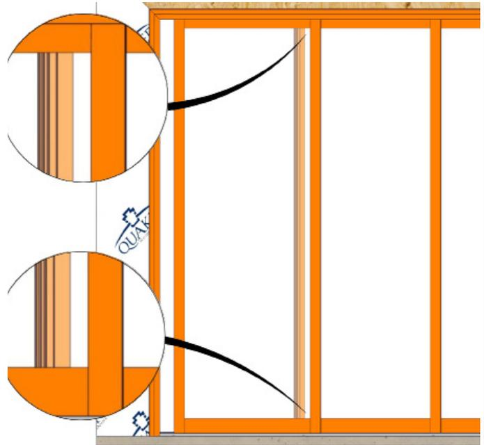
Slide each set of panels apart to check that the reveal matches at the top and bottom. Adjust rollers as needed to match reveal across panels.
