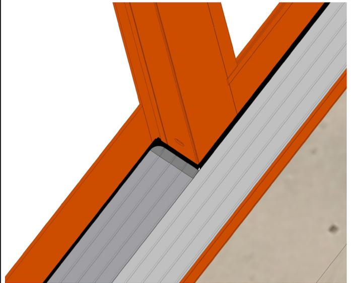
On the exterior sill cover cut out the weather strip where it meets the sill cap you just previously installed.
