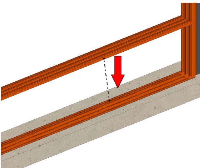
Set the sill in place, and push towards the exterior to lock in the sill to the sill pan.
