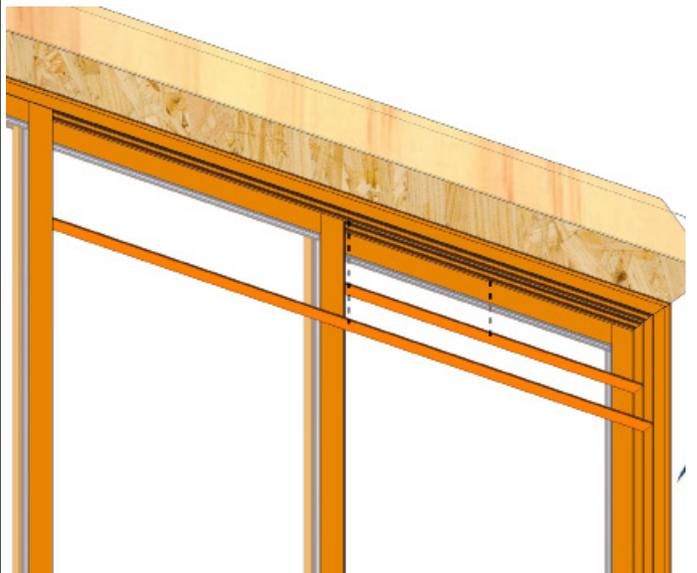
Next install the short and long header covers in the exterior and middle tracks. Trim covers to fit if needed.
