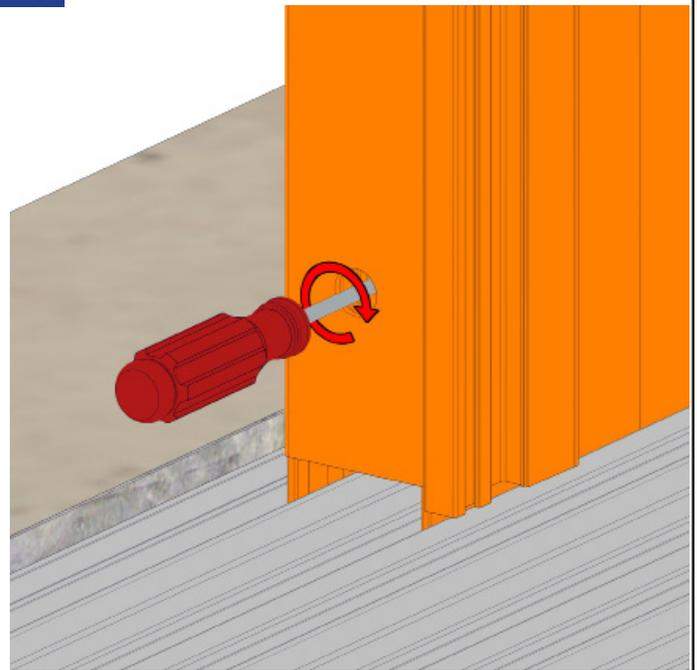
Use a #2 phillips screwdriver to engage the roller adjustment on both sides of a panel. Turn clockwise to raise the panel and provide smooth rolling. If possible, lift the panels slightly when adjusting to take pressure off the rollers. Roll panel back and forth 2-3 times to verify roller height is set.
