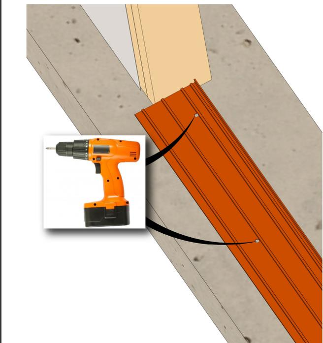
Locate second and third leg and drill holes directly behind them. Drill holes through the sill pan, 3" from each end and then 14" on center for the length of the pan, alternating between the 2 tracks. Blow out the debris on the sill pan. (Drill bit size is based off screw size)
