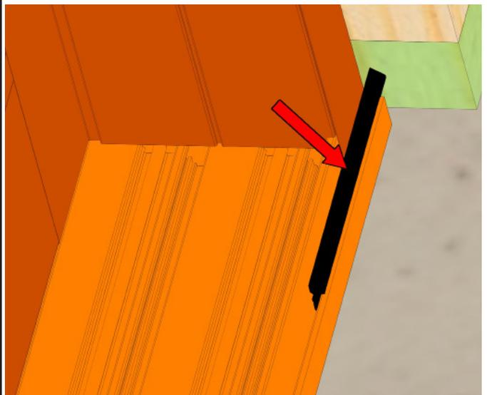
Cut a small piece of wedge gasket and place it in the center, as well as, one piece at each end.
