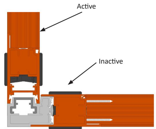
Once all the panels are installed close the panels. Make sure the inactive and active panels lock as shown above.
