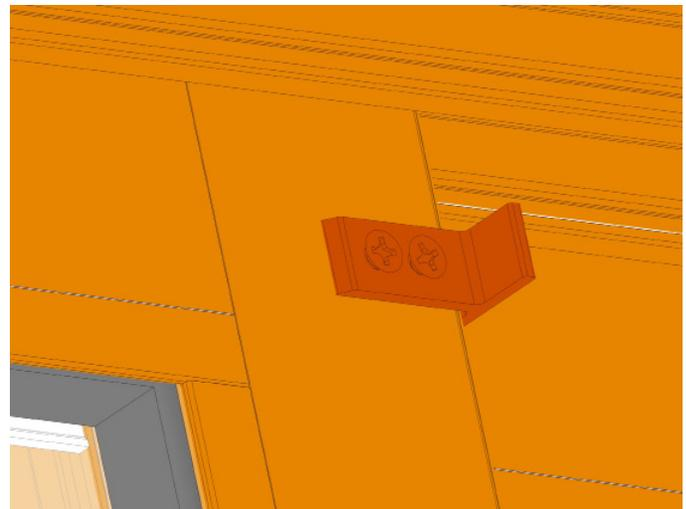
On the interior side of the middle panels, take the panel pickups (Part #: M25296-PCS) and #10 screw (Part #:MF10AX1) that is provided. Take screws and attach the pickups. Install the panel pickup where the holes are already fabricated on the interior side of the door. wd
