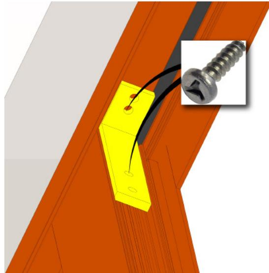
Install the tri-wing screws.
