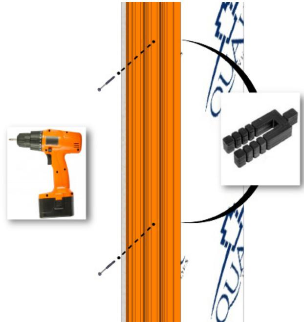
Fully fasten the screws down now to hold the frame in place. The holes through the center track of the header & jambs, typically 6" from ends and 2' on center for fasteners. Shim tight to sill pan.
