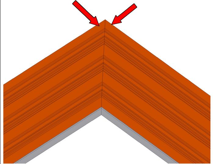
Make sure that there is less than a 1/16" gap between the 2 pieces of sill.
