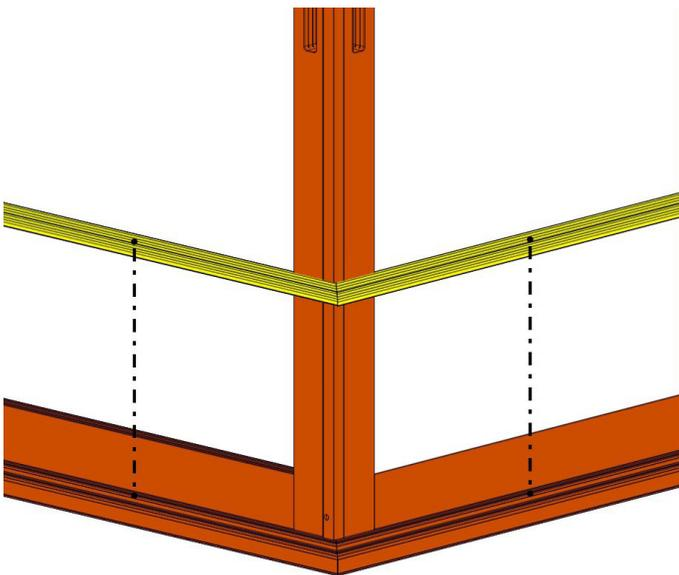
Repeat next steps for both sides. Lay out sill cover before installing, start with the sill cover closer to the interior.
