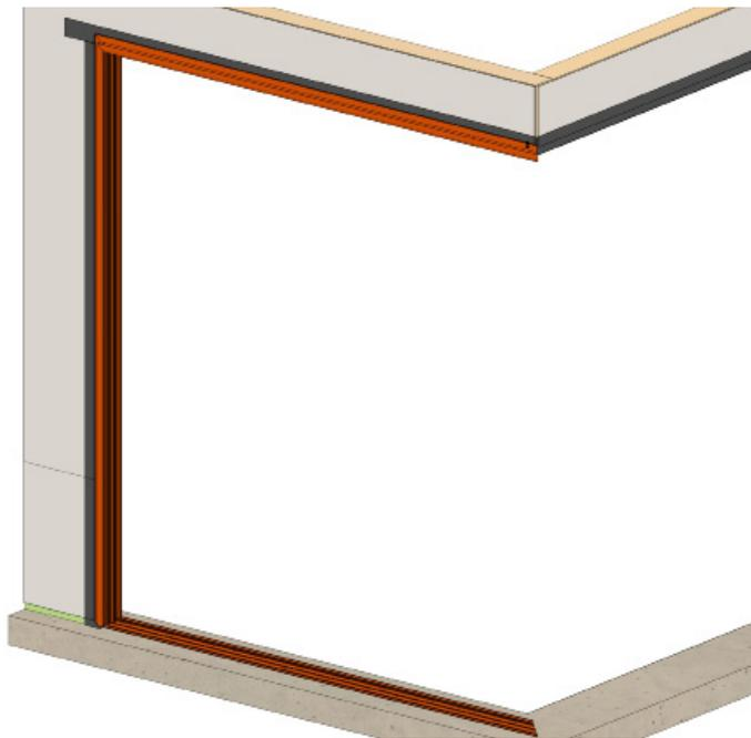
Install half the frame by sliding in the rough opening with the fin to the exterior side. Set the jamb in the sill pan so that the exterior faces of the sill pan. Measure sill pan is in line with the frame jamb.
