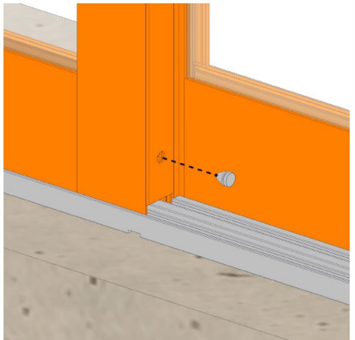
Once all panels have been adjusted install the panel bumpers (Part #: 9309K86) into each roller adjustment hole.
